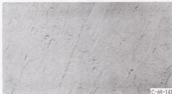
(d) After 698.2 hours at 2200° F (1204° C).
