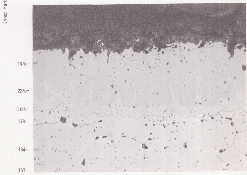
(b) Silicide coating modified with 15V - 35Mo - 35W - 15Ti. C-68-4325
