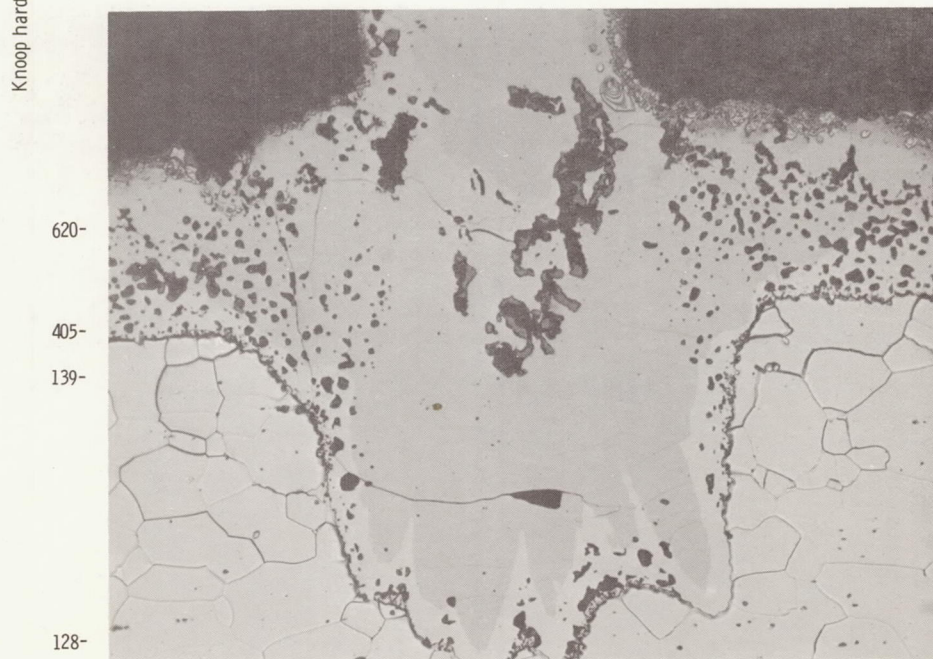
(b) Air exposed for 100 hours at 2100° F (1420° K).
