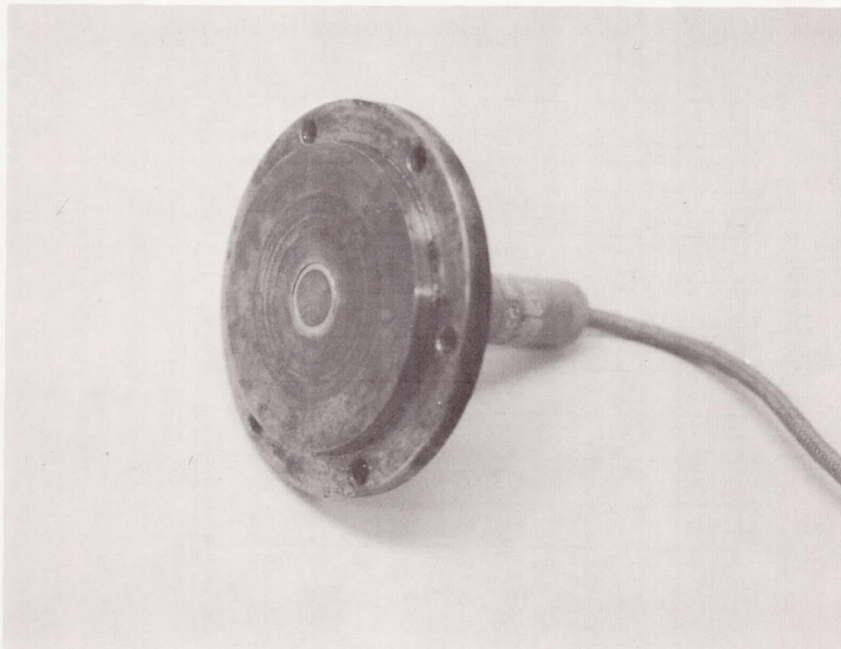
Figure 18 Microphone Used for Boundary Layer Fluctuation Measurements
