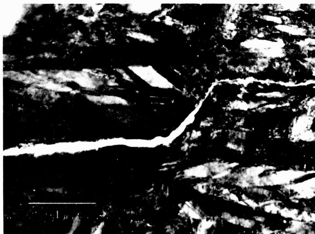
FIGURE 12. Ti-6Al-4V, STA, STRESSED IN RED N_2O_4 , SHOWING CRACK RUNNING PARALLEL TO MARTENSITE INTERFACES BATTELLE MEMORIAL INSTITUTE - COLUMBUS LABORATORIES
