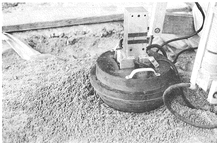
Fig. 35 View of Final Resting Position of Heavy Cone - Dry, Dense Colorado River Sand
