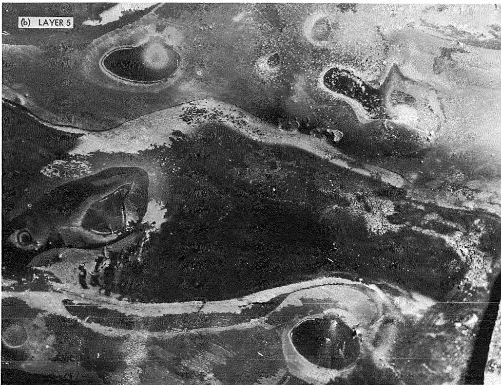
Fig. 172. Typical deterioration of separator—Surveyor main battery
