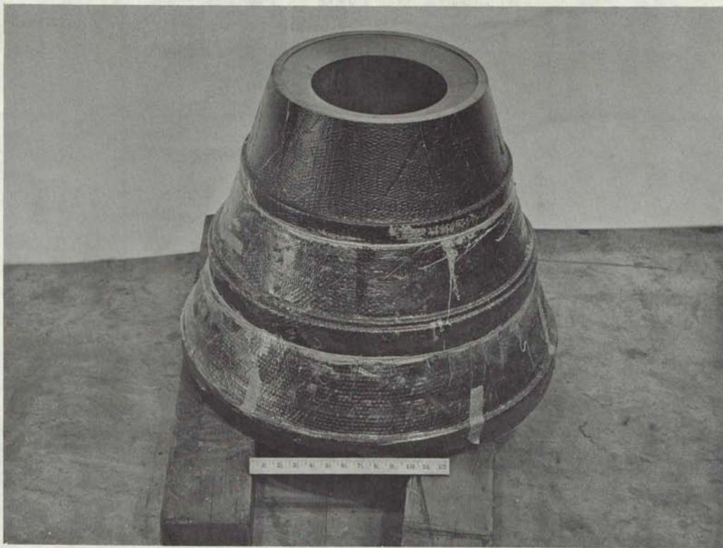
Figure 128. Nozzle No. 2 Assembled Exit Cone Tiers
