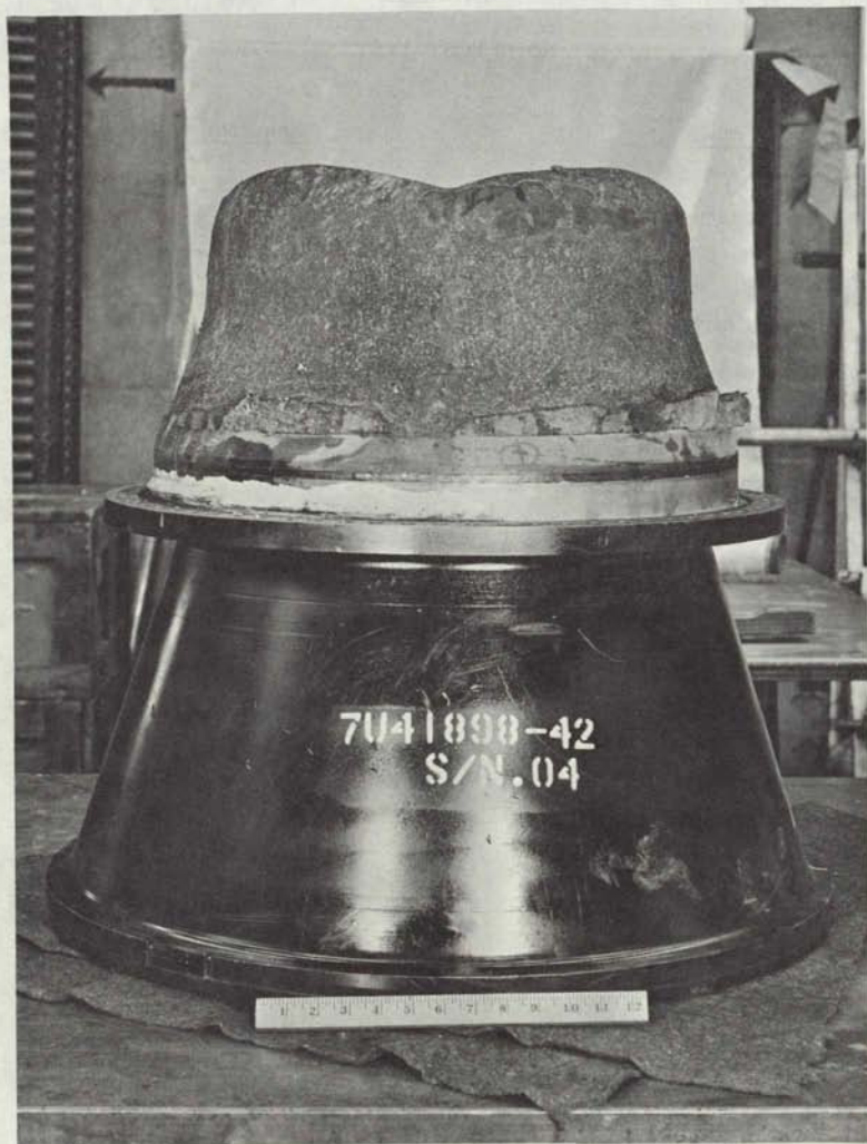
Figure 189. Nozzle No. 4 Submerged Liner
