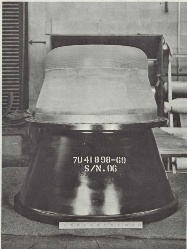
Figure 115. Nozzle No. 6 Before Test (View A)
