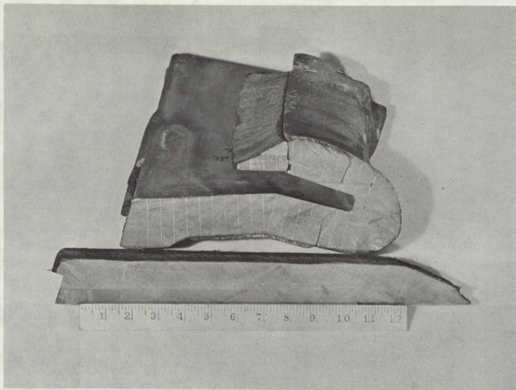
Figure 193. Sectioned Nozzle No. 4 Submerged and Exit Cone Liners
