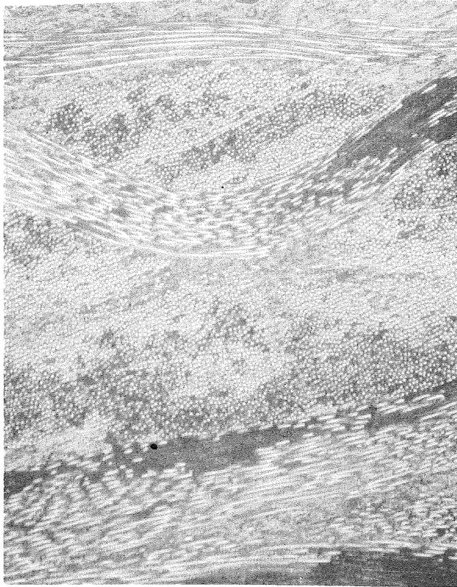
Figure E-4. Photomicrograph of MNP A-Type Polyimide Silica Laminate 24.9% Resin, 60 X Magnification
