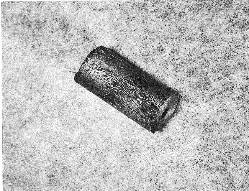
Figure E-6. PEET Specimen Tungsten Reinforced A-Type Polyimide Prepared by Electron Discharge Milling
