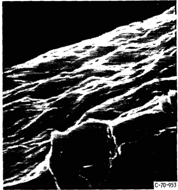
(c) Tensile fracture surface of wrought aluminum foil material. X2000.
