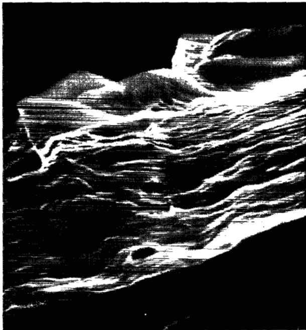
(b) Tensile fracture surface of electroformed aluminum liner material. X2000.
