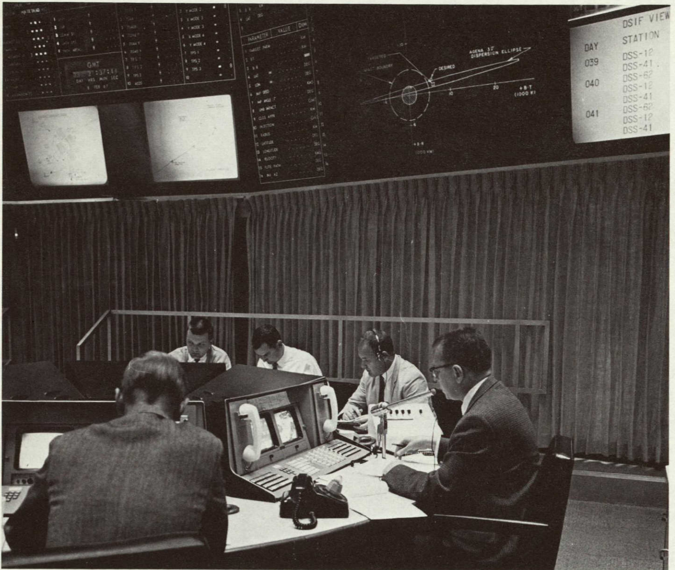
Fig. 23. Circular console in the SFOF DSN operations area. This position was used for launch and flight operations commentary to all NASA facilities
