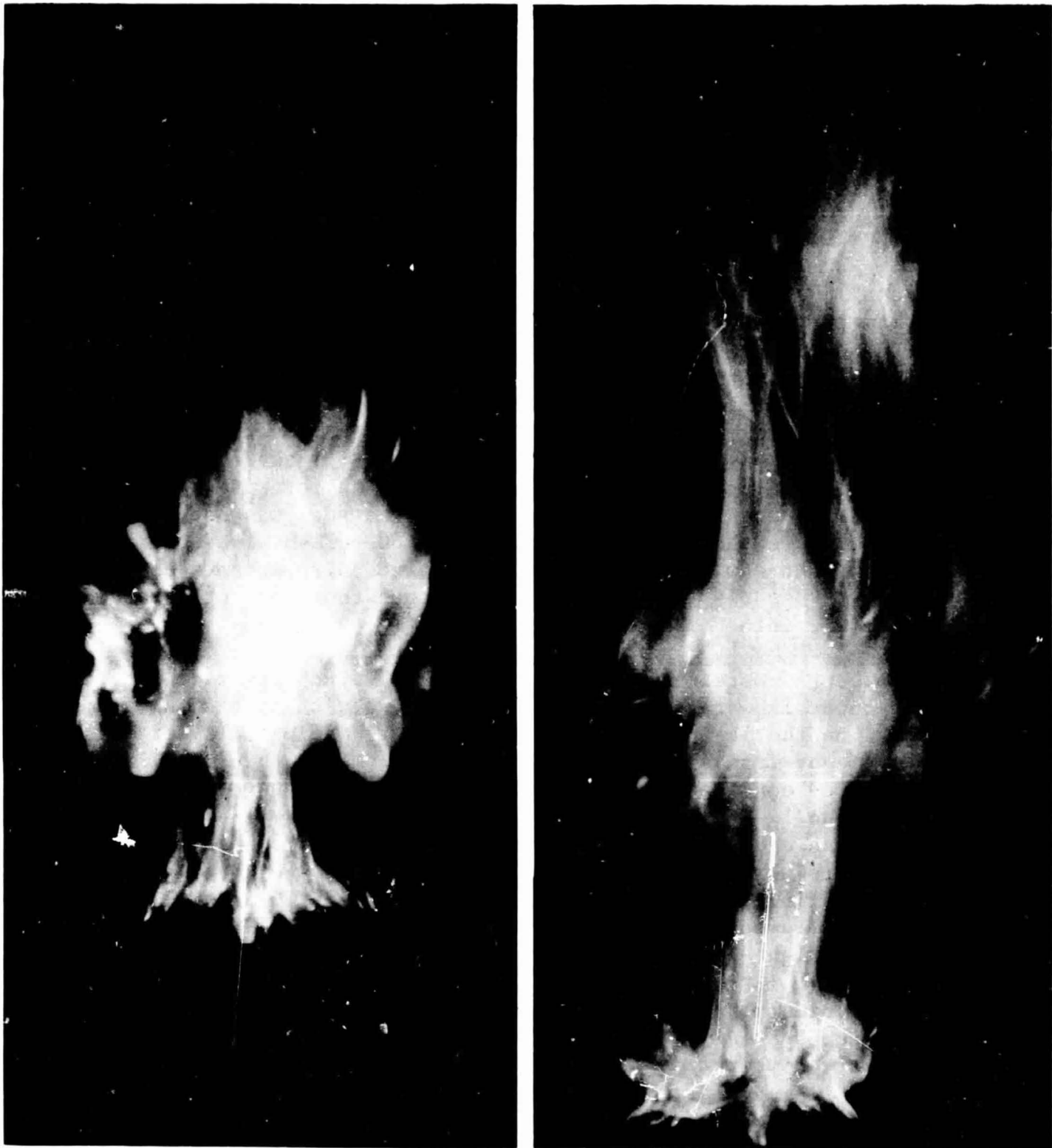
FIGURE 4. - Two Views of a Hydrogen Diffusion Flame on a 12-Inch Stack, Flow Rate = 0.66 cfs.
