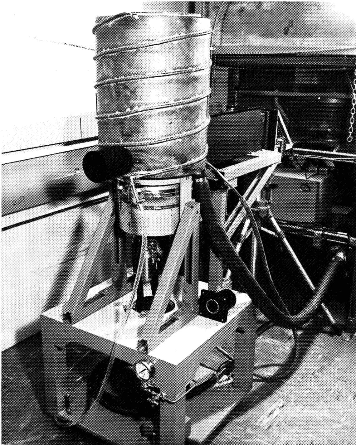
Figure 18.4 Lamp with protective enclosure in place
