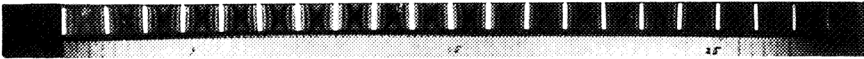
Figure 9.2 Fringe pattern from a time-average hologram of a cantilevered beam 30 in. long vibrating in its twenty-first mode (10, 121 Hz)
