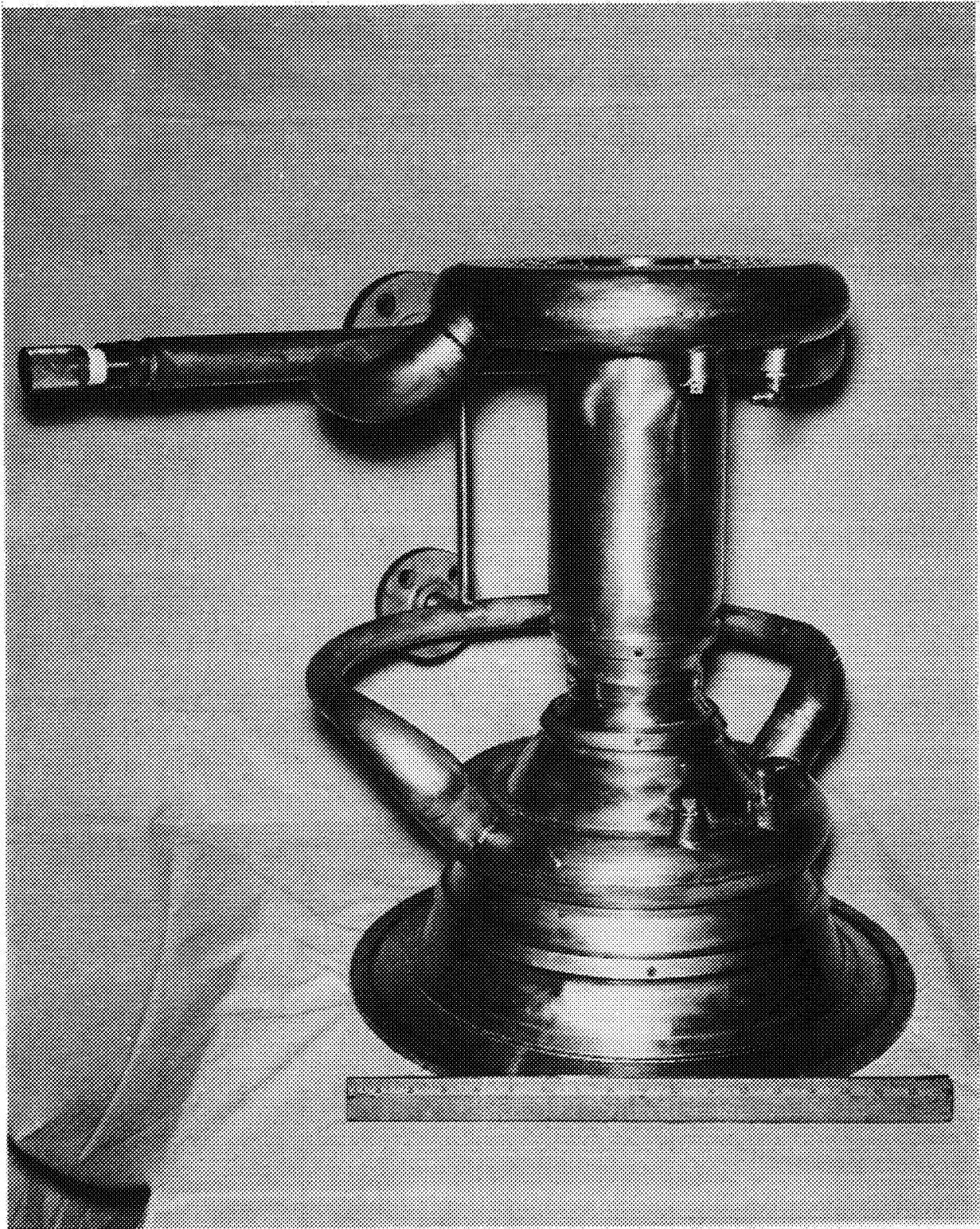
Figure 25. Thrust Chamber with Plumbing Attached
