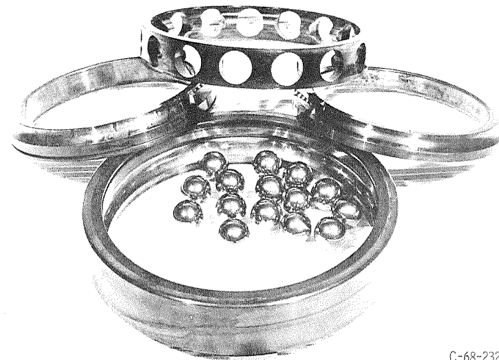
Figure 11. - Unfailed 120-mm angular-contact ball bearing run with synthesized hydrocarbon oil containing substituted organic phosphonate. Material, AISI M-50 steel; thrust load, 5800 lb; speed, 12,000 rpm; temperature, 600° F; low-oxygen environment; running time, 500 hrs. ( 360 \times 10^6 inner-race revolutions).
