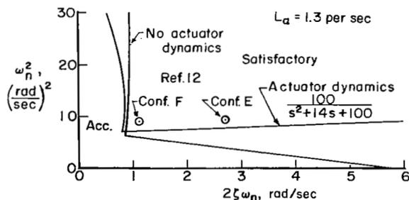
Figure 16.- Effect of actuator dynamics on attitude-control boundaries computed by using first-level pilot model (no lead) with  $L_\alpha = 1.3$  per sec.
