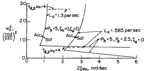
Figure 11.- Comparison of altitude-control boundaries computed by using first-level pilot model for two values of  $L_{\alpha}$ . (Values of  $P_h$  and  $P_{\alpha}$  are in seconds;  $T_{\theta,2}\omega_n$  is in radians.)
