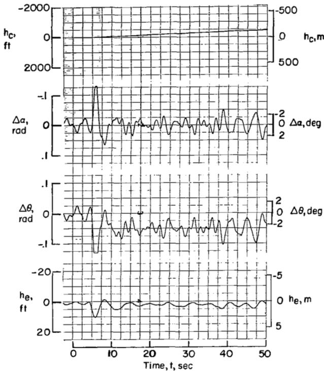
Figure 18.- Landing-approach time history computed by using second-level multiloop pilot model with remnant.  $\omega_n = 2.5$  rad/sec;  $\zeta = 0.32$ . (To facilitate comparison with fig. 17,  $\Delta\alpha$  and  $\Delta\theta$  are given in degrees as well as radians.)
