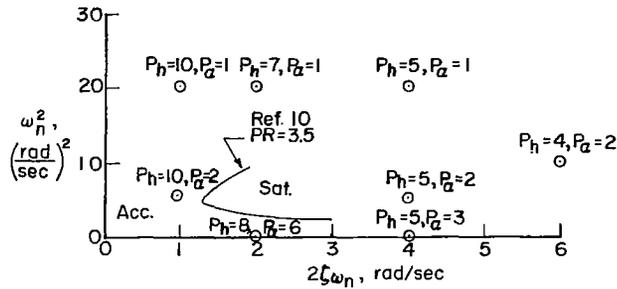
Figure 4.- Results of trial-and-error procedure for obtaining best closed-loop system response for altitude control, with first-level pilot model used. (Values of  $P_h$  and  $P_\alpha$  are in seconds; the pilot-rating boundary from ref. 10 is presented for comparison.)
