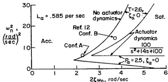
Figure 15.- Effect of actuator dynamics on attitude-control boundaries computed by using first-level pilot model (no lead) with  $L_\alpha = 0.585$  per sec. (Values of  $T$  and  $P_\alpha$  are in seconds.)
