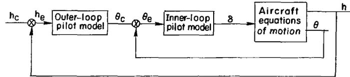
Figure 1.- Block diagram of a typical multiloop system.
