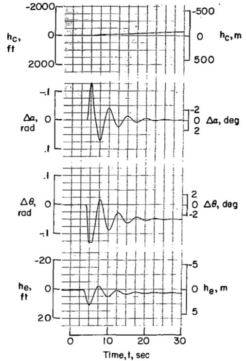
Figure 19.- Landing-approach time history computed by using second-level multiloop pilot model without remnant.  $\omega_n = 2.5$  rad/sec;  $\zeta = 0.32$ . (To facilitate comparison with fig. 17,  $\Delta\alpha$  and  $\Delta\theta$  are given in degrees as well as radians.)
