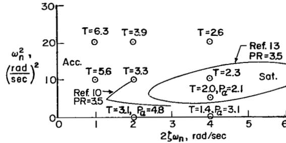
Figure 5.- Results of trial-and-error procedure for obtaining best closed-loop system response for attitude control, with first-level pilot model used. (Values of  $T$  and  $P_\alpha$  are in seconds; the pilot-rating boundaries from refs. 10 and 13 are presented for comparison.)
