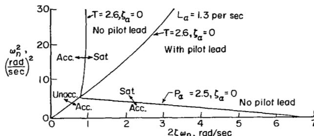
Figure 14.- Comparison of attitude-control boundaries computed by using first-level pilot model (no lead) and second-level pilot model (lead). (Values of  $T$  and  $P_\alpha$  are in seconds.)
