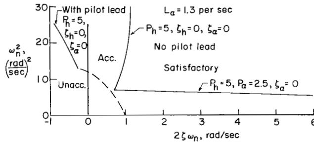
Figure 13.- Comparison of altitude-control boundaries computed by using first-level pilot model (no lead) and second-level pilot model (lead). (Values of  $P_h$  and  $P_\alpha$  are in seconds.)
