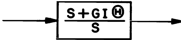
Figure 28.- Integral plus proportional compensation
