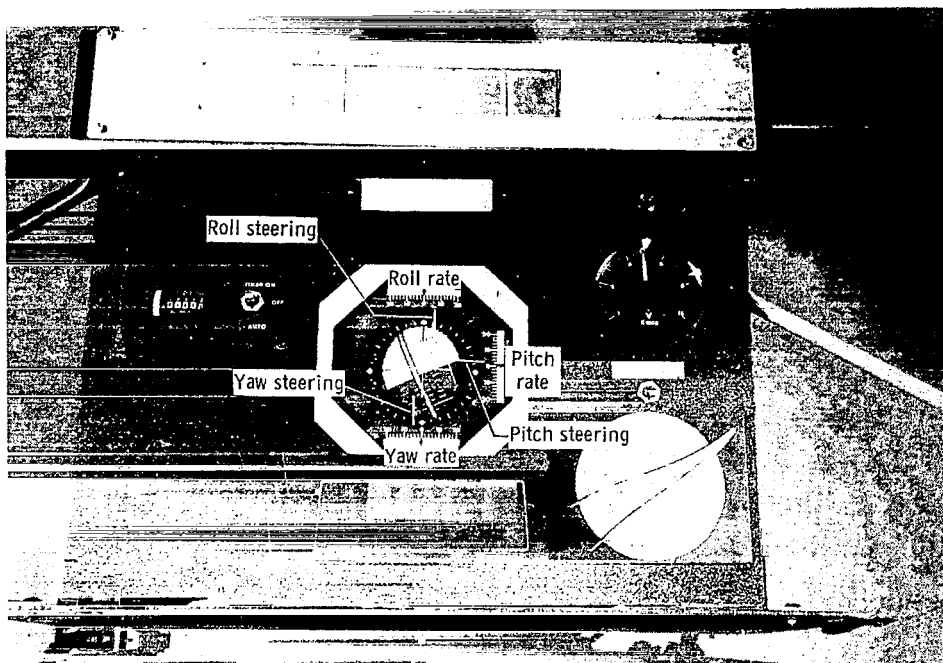
Figure 10.- A pilot's view of the three-axis 8-ball in unmasked configuration.
