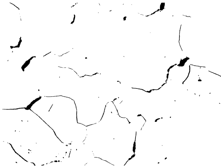
(b) Powder-metallurgy (PM) rhenium after 2 percent total elongation (rupture).
