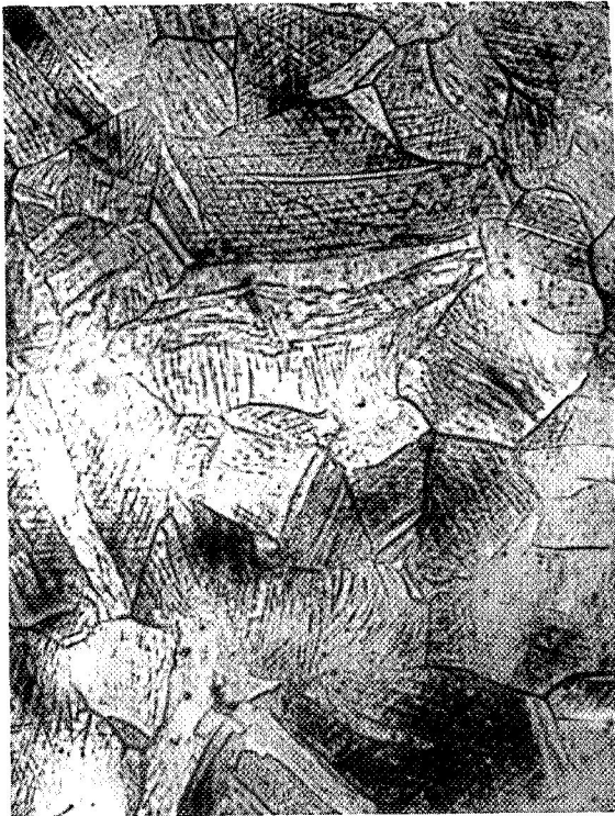
FIGURE 7- MICROSTRUCTURE OF MP35N MULTIPHASE ALLOY (49% C.W. & AGED) 1.0-INCH DIAMETER BAR
