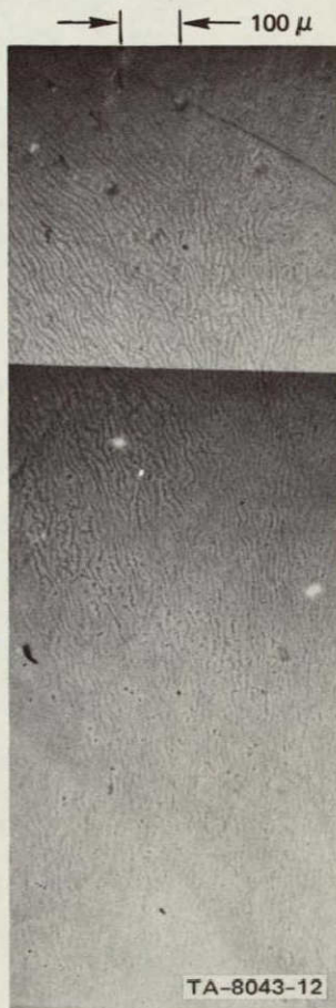
FIGURE 30 FLUX DISTRIBUTION AT THE SAMPLE EDGE. Lines of high flux density show a quasi-intermediate state structure.
