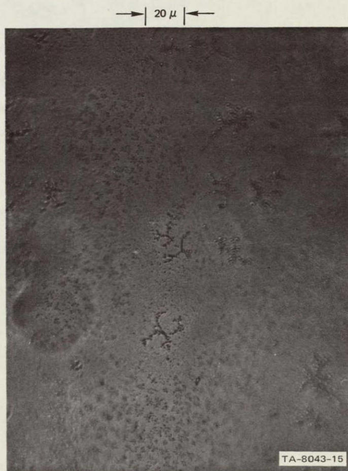
FIGURE 33 FLUX DISTRIBUTION AT CENTER OF SAMPLE. The regions of high flux density have a structure that is not fully resolvable in this micrograph.
