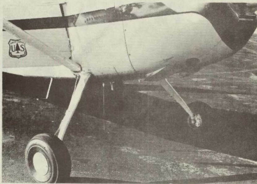
Figure 12: Antenna system installed in the landing gear access holes of a Cessna 185
