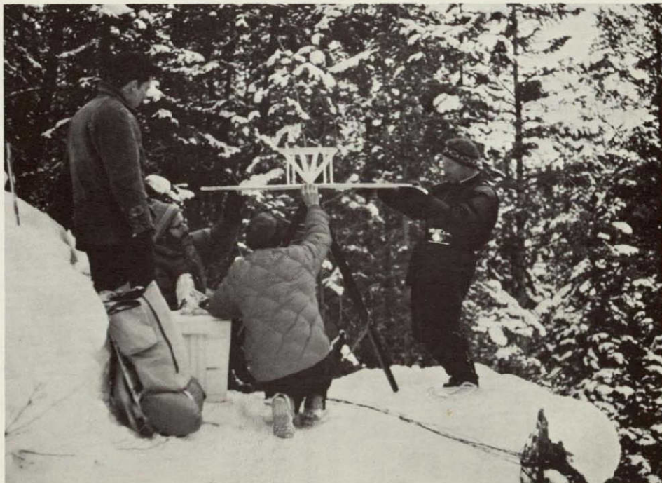
Plate 6: Setting up the antenna for the satellite data collection equipment
