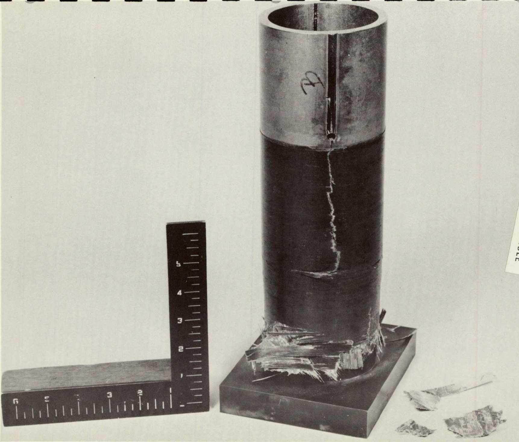
Figure 5-4 Side View of Failed Subelement Number 1
