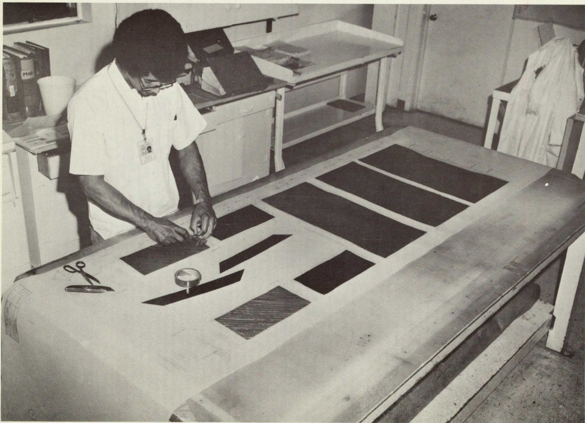
Figure 3-5 Mylar Layup Template
