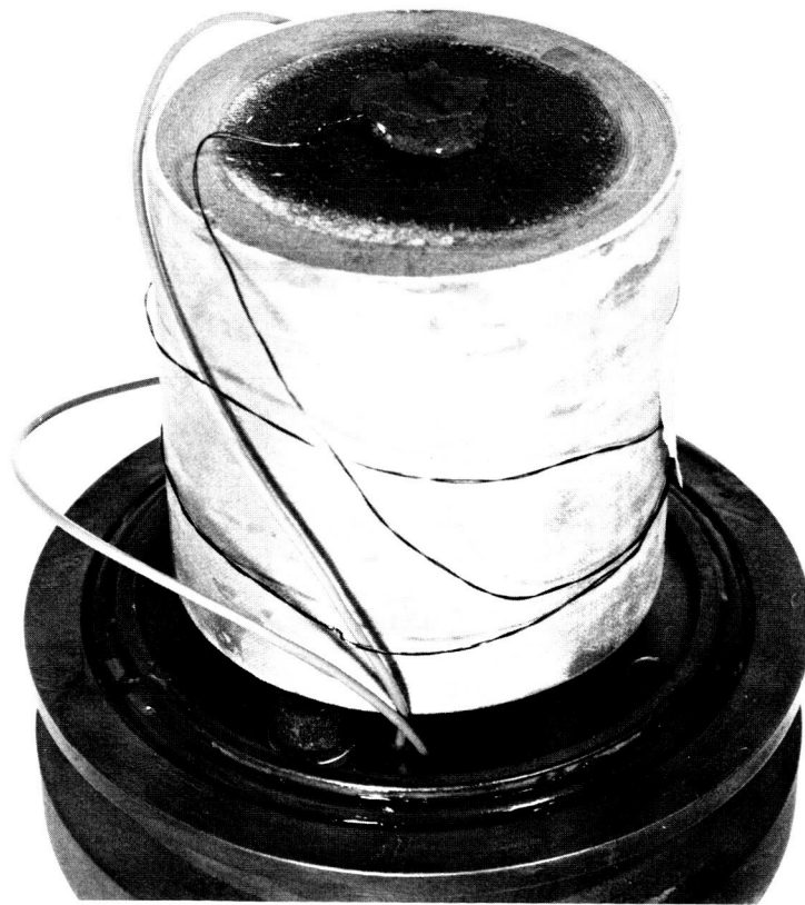
Fig. 5. Igniter end-burner propellant charge, Test 4
