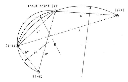
Since any radius in this sketch may be infinite, it is more convenient to work with halfcurvatures (h, h', and  $h_{av}$ ). Let  $h = \frac{1}{2r}$ ,  $h' = \frac{1}{2r'}$ , and  $h_{av} = \frac{1}{2R}$ . Then,
