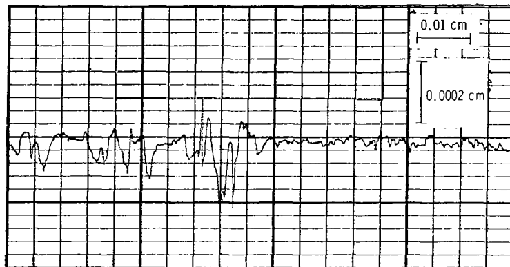
Figure 4. - Photomicrograph and surface profile of wear track of nickel rider on tungsten disk. (The micrograph and the profile are not necessarily of the same point on the disk. Also, note that the vertical scale has been expanded relative to that of fig. 3.)
