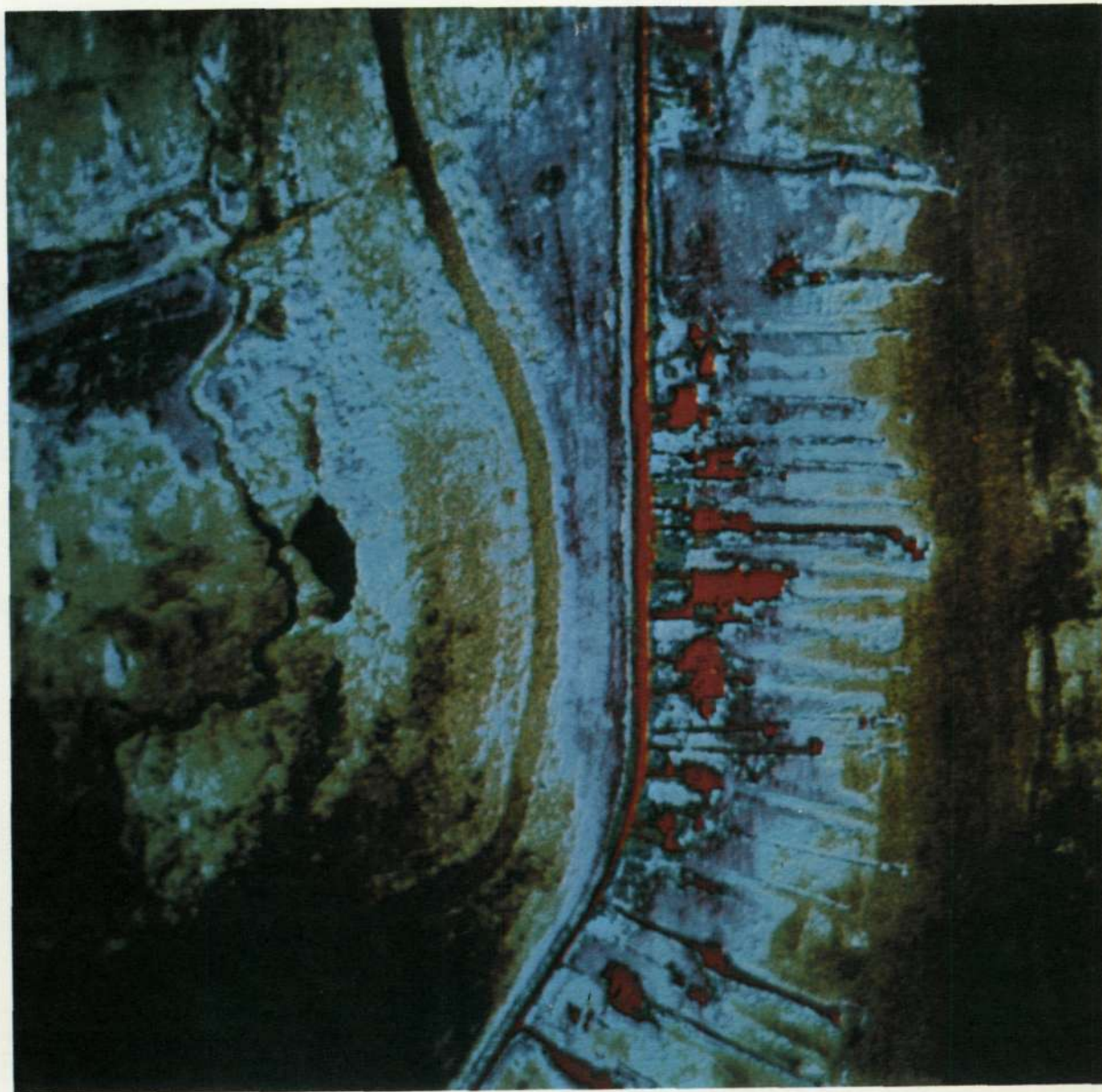
Figure 13.- This photograph was acquired from the display of the I 2 S Multiband Camera Film Viewer (MCFV) which electronically processed the 2402 black and white film exposed by the KA-62 multiband cameras of the test site. This particular camera recorded the green band. False color assignment and edge enhancement have been accomplished for this band as seen here.
