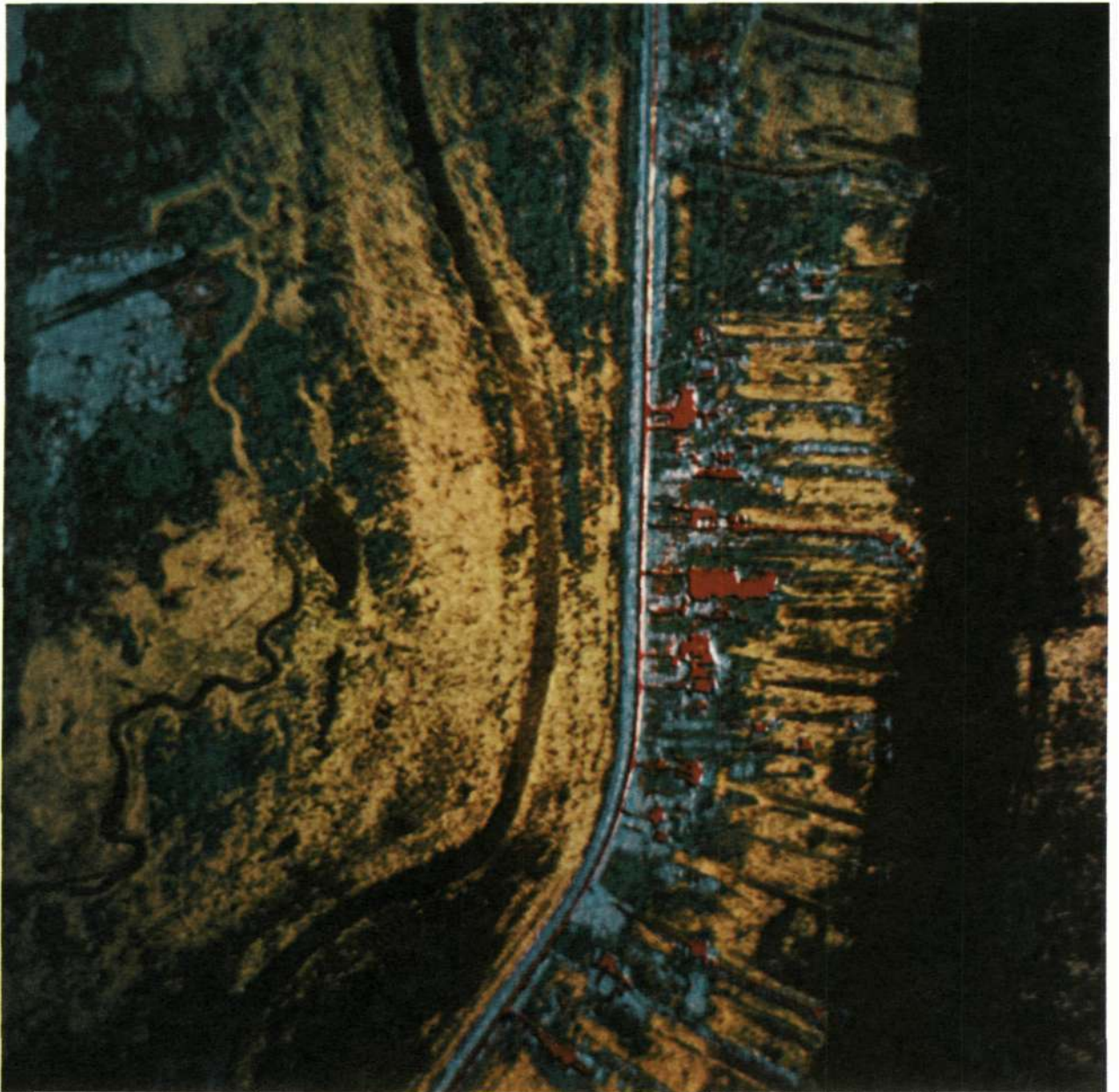
Figure 14.- This photograph, acquired by the same means as that seen in Figure 13, was derived from the KA-62 multiband camera that exposed the 2402 film in the red band.
