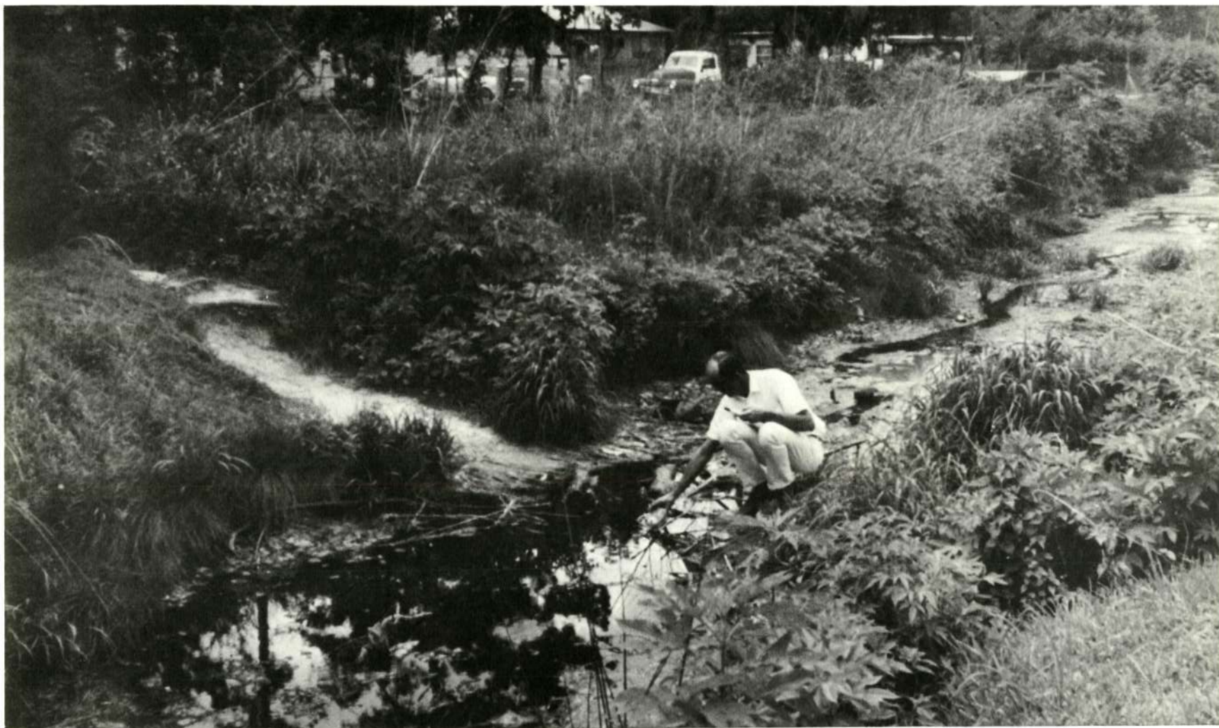
Figure 7.- A laboratory technician is seen collecting water samples from one of ten test sites near Little York Road in north Houston, Texas. These samples taken at the time of overflight were surveyed for physical, chemical, microbiological and entomological characteristics.
