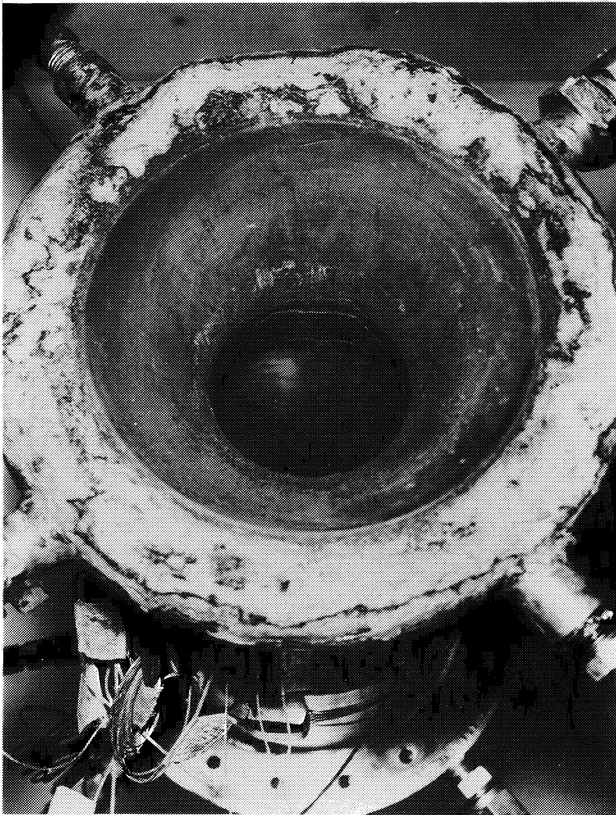
Figure 56. Posttest No. 14 Exit End Showing Carbon Deposit
