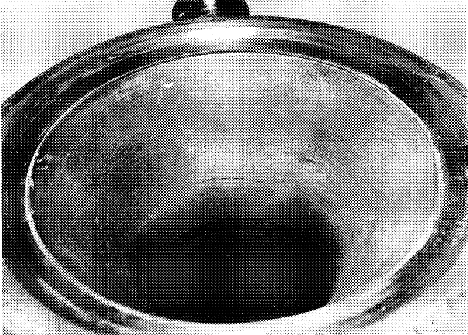
Figure 39. SN 2 Showing Delamination in Exit Section
