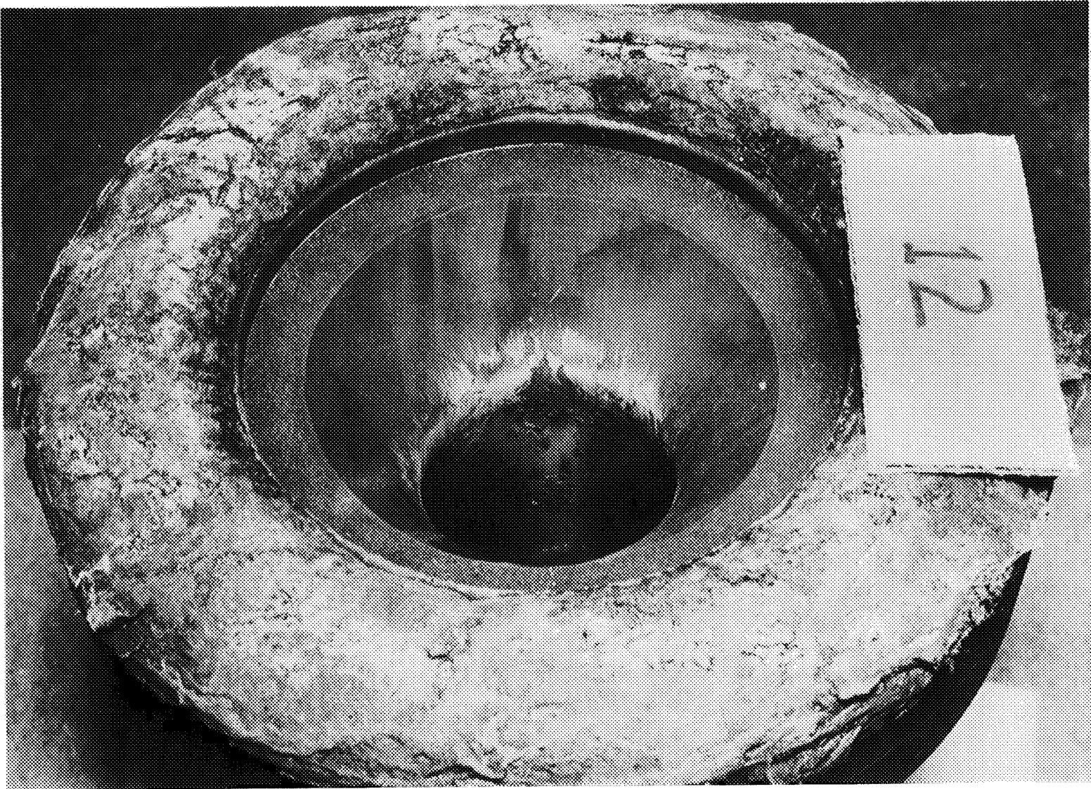
Figure 51. Graphite-Lined Workhorse Chamber, Posttest
