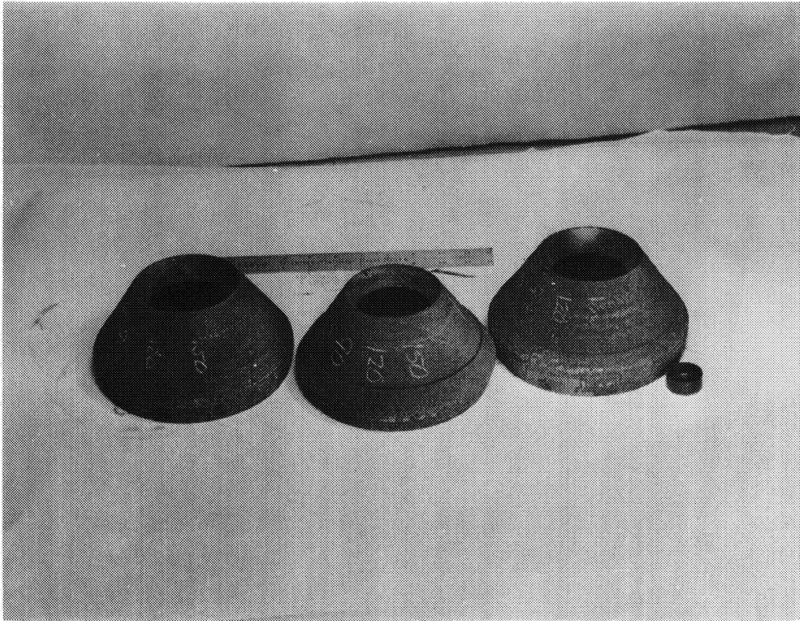
Figure 35. Exit Segments Bonded, Cured and Rough Machined
