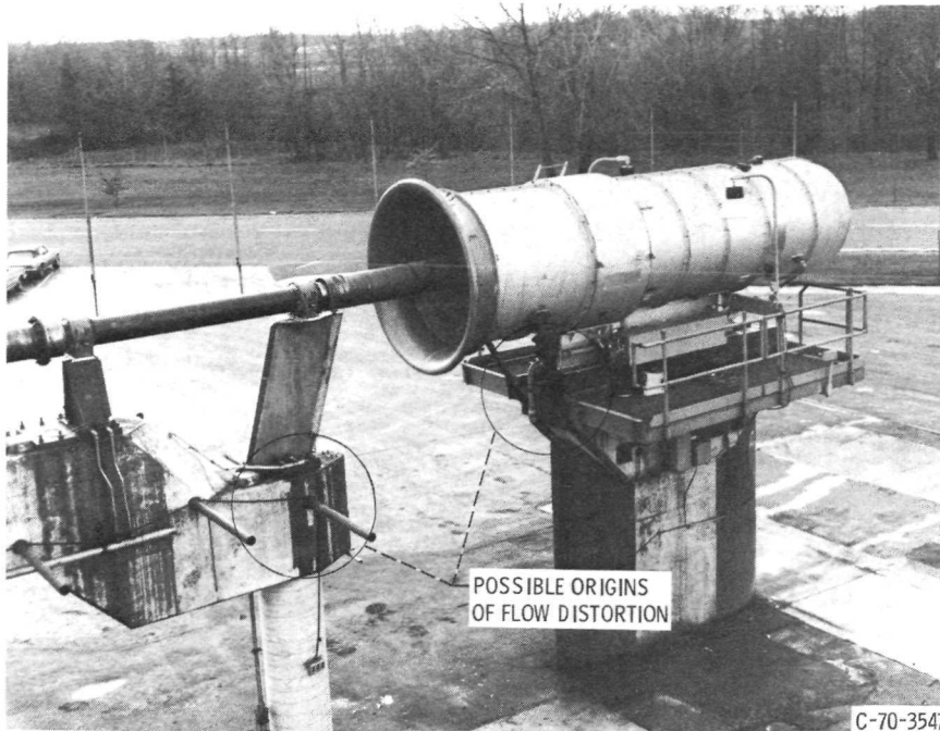
Figure 18. - Closeup view of structures believed to cause inlet flow distortion.
