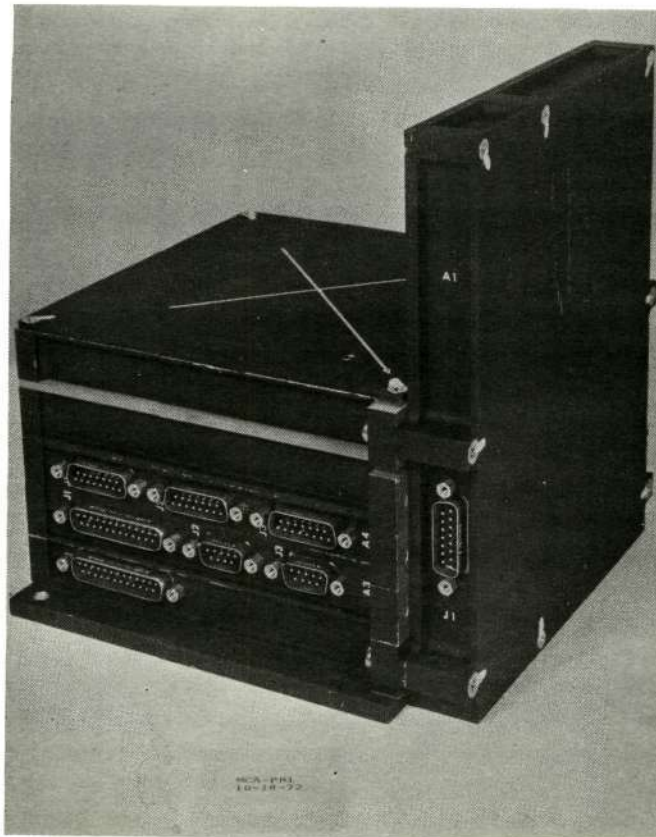
Control Logic Assembly of MCA PR1
