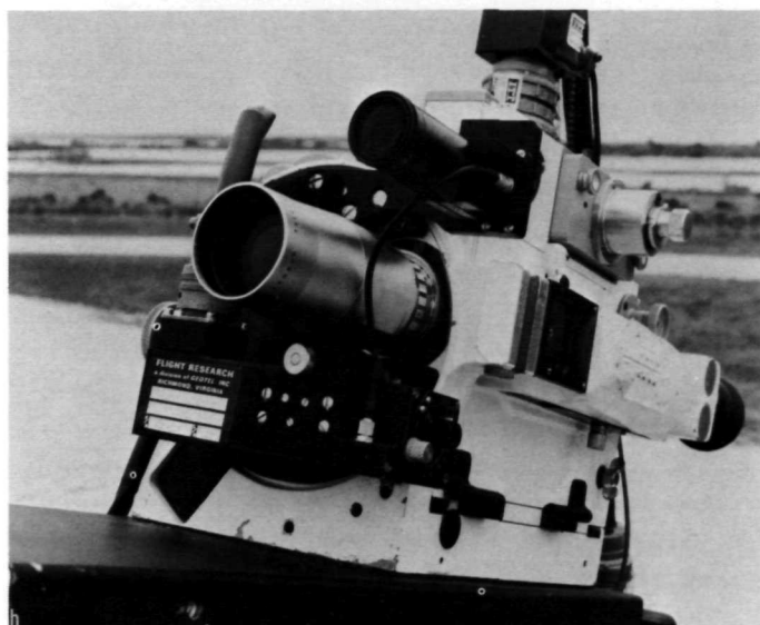
FIGURE 40.—Views of remote engineering data cameras installed at a photographic site at Launch Complex 39A at Kennedy Space Center. Figure 40(b) shows a camera with sun cover and shield removed. The silver finish barrel contains the main lens of the camera. The small black barrel holds the sensor lens that is used to adjust the main lens aperture in response to the instantaneous light level.
