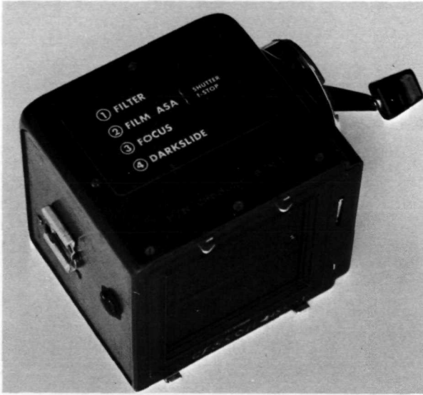
FIGURE 6.—The first version of the Hasselblad camera, as modified by NASA for use in the Mercury Program. The body is shown without lens and magazine. The magazine used is that of figure 4. (Camera courtesy Smithsonian Institution.)
