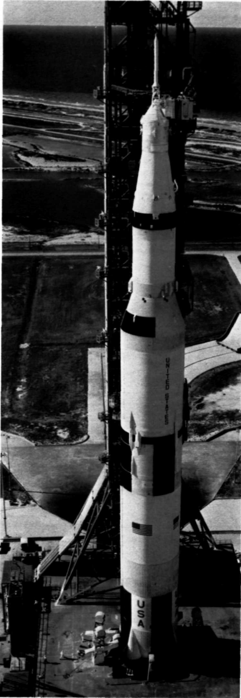
FIGURE 42. —This photograph of the Saturn vehicle nearing liftoff shows the launch umbilical tower immediately behind the vehicle. Note on the left the camera platforms on which the engineering data cameras are installed to record various events during liftoff procedure. Note also the cameras near the base of the vehicle for direct recording of the engines during the initial stages of operation.
