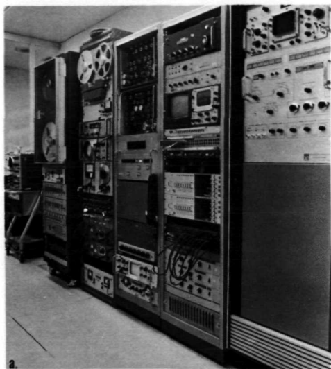
FIGURE 54.—The communication and photo-optical equipment used for reconstruction of color photographs from ATS III is shown (a), with magnetic tape units used for intermediate storage of picture information (b), and the electro-optical reconstruction equipment (c), which contains a very precise color cathode ray tube. The film holder is on the right of the cabinet.
