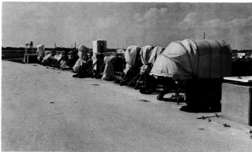
FIGURE 18.—Site 4 at Launch Complex 39A, Kennedy Space Center, with cameras installed and covered for protection until launch operations.
