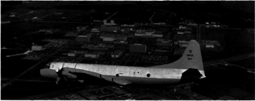
FIGURE 14.—The NASA flying camera platform and NP 3A Aircraft, a modified Lockheed Electra is used by NASA for the Earth Resources Observation Program. It is shown against the background of the Manned Spacecraft Center at Houston.
