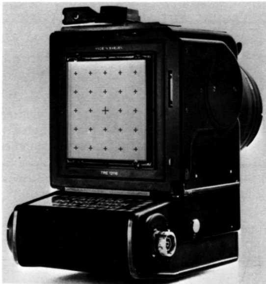
FIGURE 10.—A photograph of the Lunar Data Camera showing the reseau grid plate at the focal plane of the camera body. (Paillard, Inc.)
