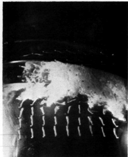
FIGURE 34.—A photograph taken by a camera focused axially along the pump impeller. It shows the cavitation of the leading edge of the impeller toward the lower part of the picture. This picture was made from a single frame of the 35-mm camera. The perforations and framing marks have been cropped off.
