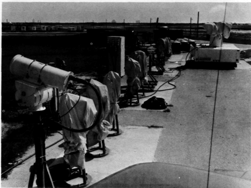
FIGURE 19.—Site 5 at Launch Complex 39A at the Kennedy Space Center, showing equipment as set up and covered until a countdown and liftoff. A large remote-controlled tracking camera appears on the trailer. Smaller cameras for recording individual events are mounted in fixed stands with known coordinate references.
