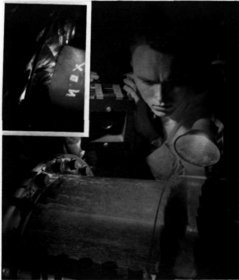
FIGURE 29.—In the test segment of the facility, a clear glass or plastic cylinder is used to inspect behavior at high speeds. This picture shows the test section and the lighting and camera arrangement. The inset shows a single frame of the motion pictures which give apparent still pictures of the pump blades, even when the blades are moving at very high speeds.
