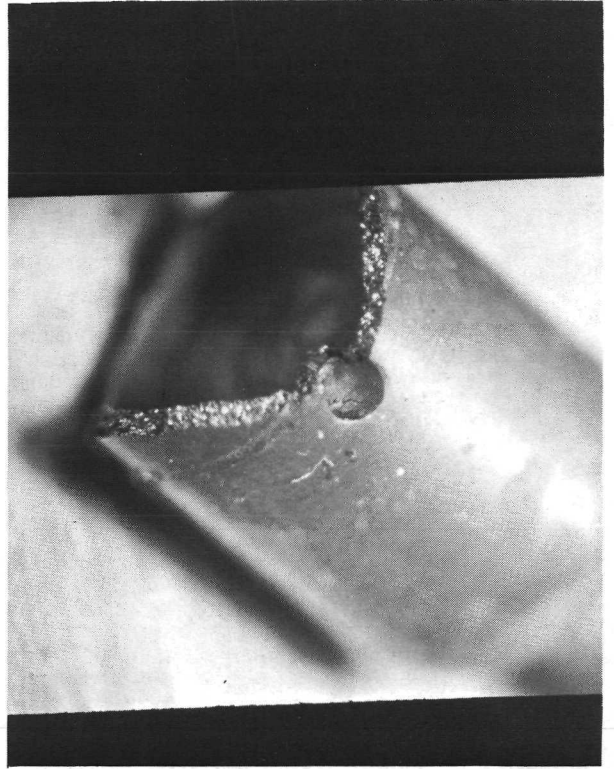
(b) End cap of fuel pin after point impact.
