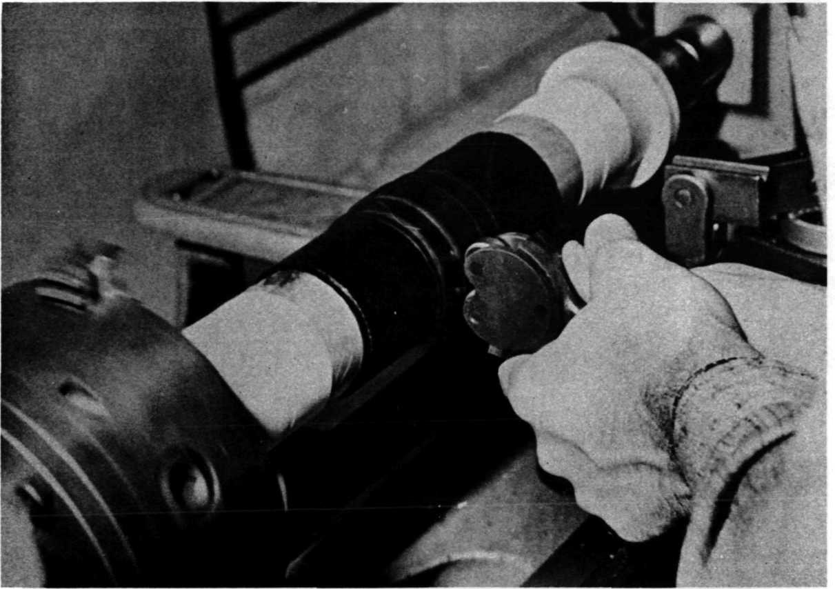
Figure 39. Rolling on the tread cover.
