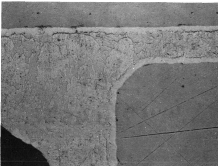
FIGURE 5. PHOTOMICROGRAPH OF TYPICAL BAg18 BRAZE JOINT FILLET AREA (Test No. 3) Magnification: 250X
