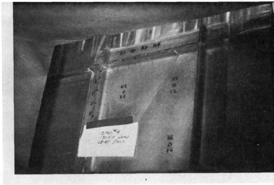
FIGURE 8A- PANEL 4 UNIAXIAL LOAD FRONT SURFACE
