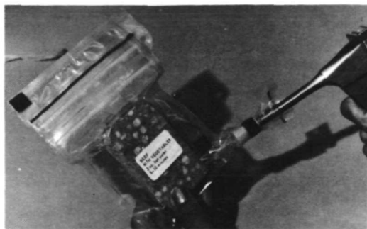
Fig. 1—Apollo rehydratable solid/semisolid food package showing spacecraft water dispenser inserted.
