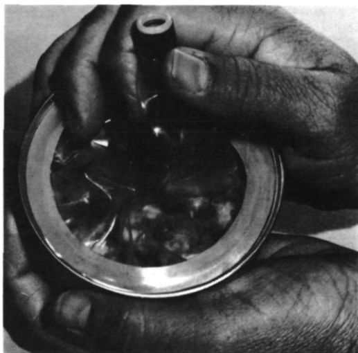
Fig. 2—Full-panel pull-out space food can fitted with flexible inner cover and 1-way spring-loaded valve for food rehydration.
