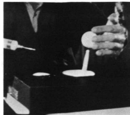
Fig. 12— GLOBULE rebounding from surface of milk in container in null gravity rapidly forms a perfect sphere (1/64-sec exposure frame from motion picture film)
