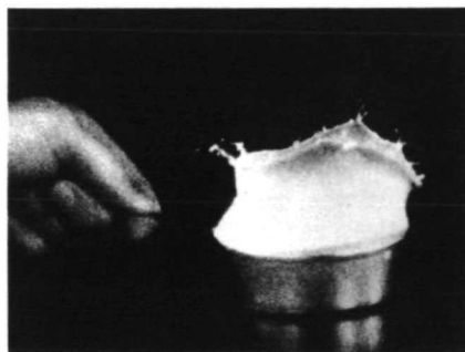
Fig. 13— UPWARD AND OUTWARD SPLASH occurs when a spoon strikes the surface of milk in a container in normal gravity (1/500-sec exposure frame from motion picture film)
