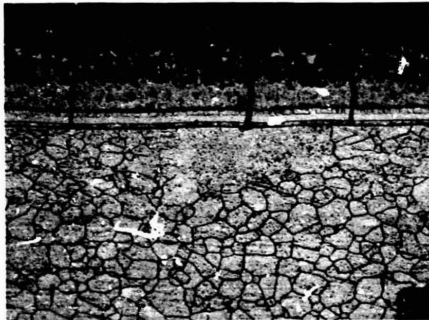
FIGURE 37. CRACK CONTAMINATION IN C129Y AND FS85 AFTER THREE DYNAMIC EXPOSURE CYCLES (RUN 11)
