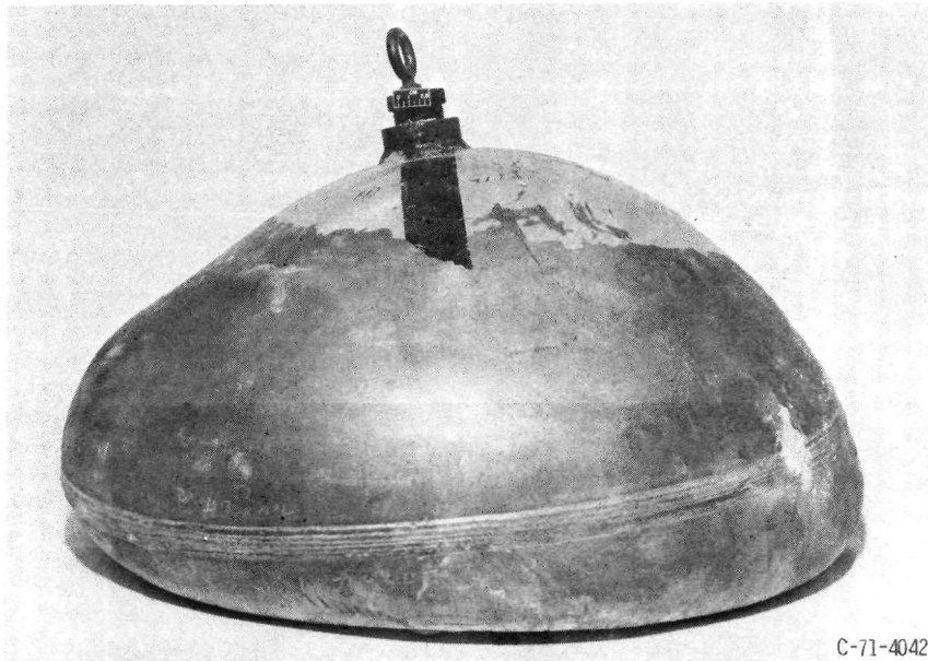
Figure 17(b). - Nuclear containment system - after impact at 1055 ft/sec.
