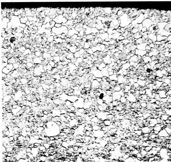
(a) T-111 capsule wall near bottom weld; heated with TZM.
