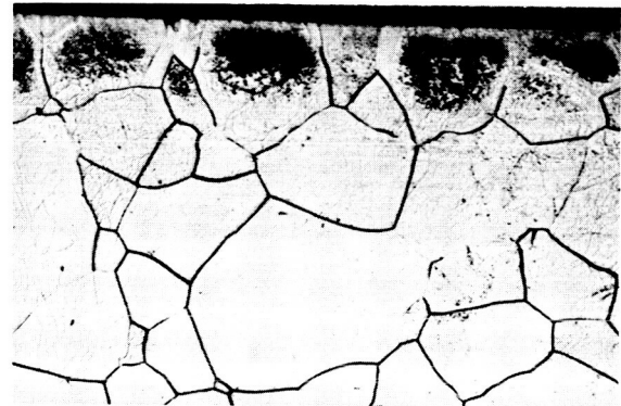
(b) T-111 capsule sidewall about 0.6 centimeter above weld.
