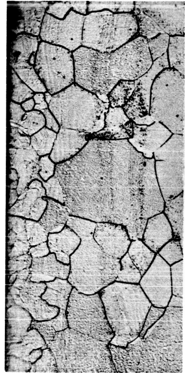
(b) T-111 capsule sidewall about 0.6 centimeter above weld.
