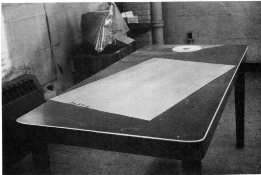
Creep Flattened Sheet - 0.5% Flatness
