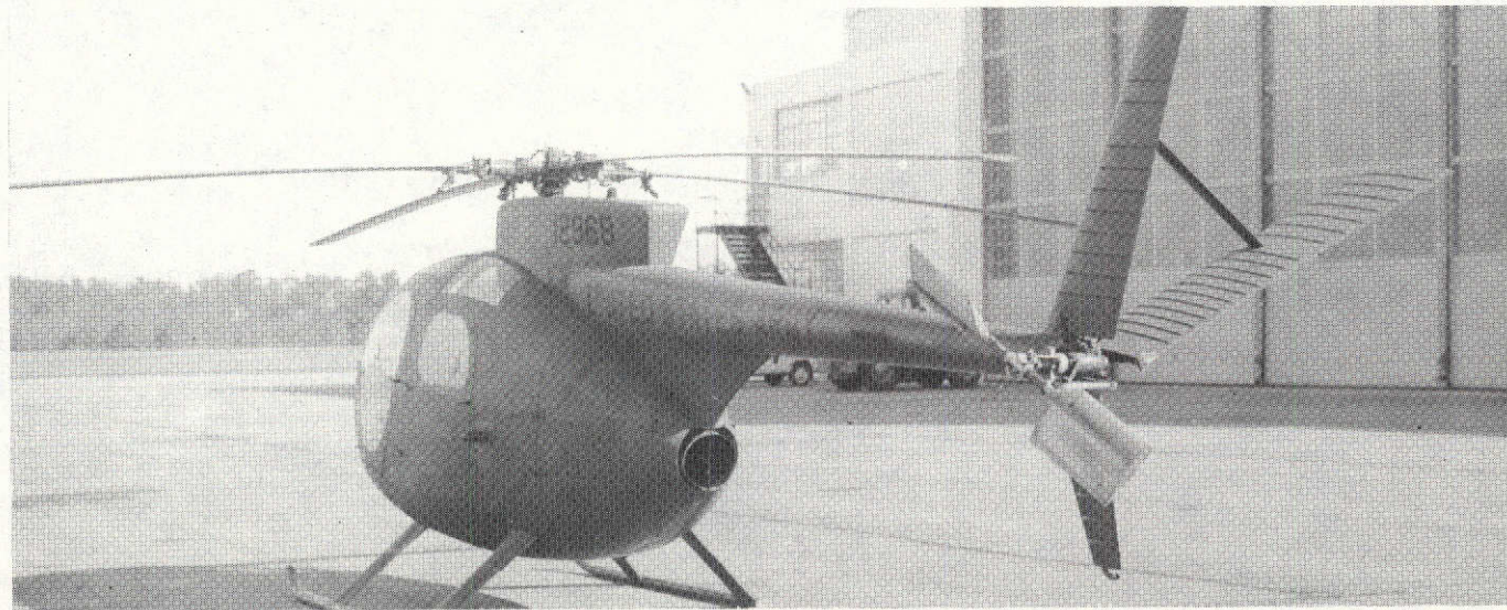
(b) Two-blade wide chord tail rotor; configuration C.
