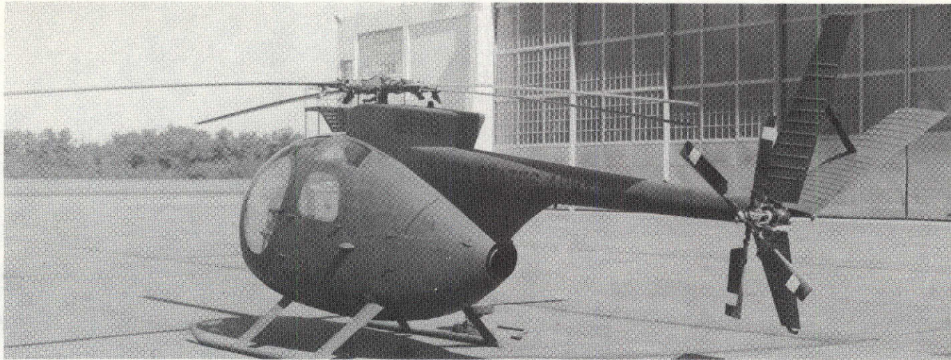
(a) Four-blade tail rotor; configuration B.
