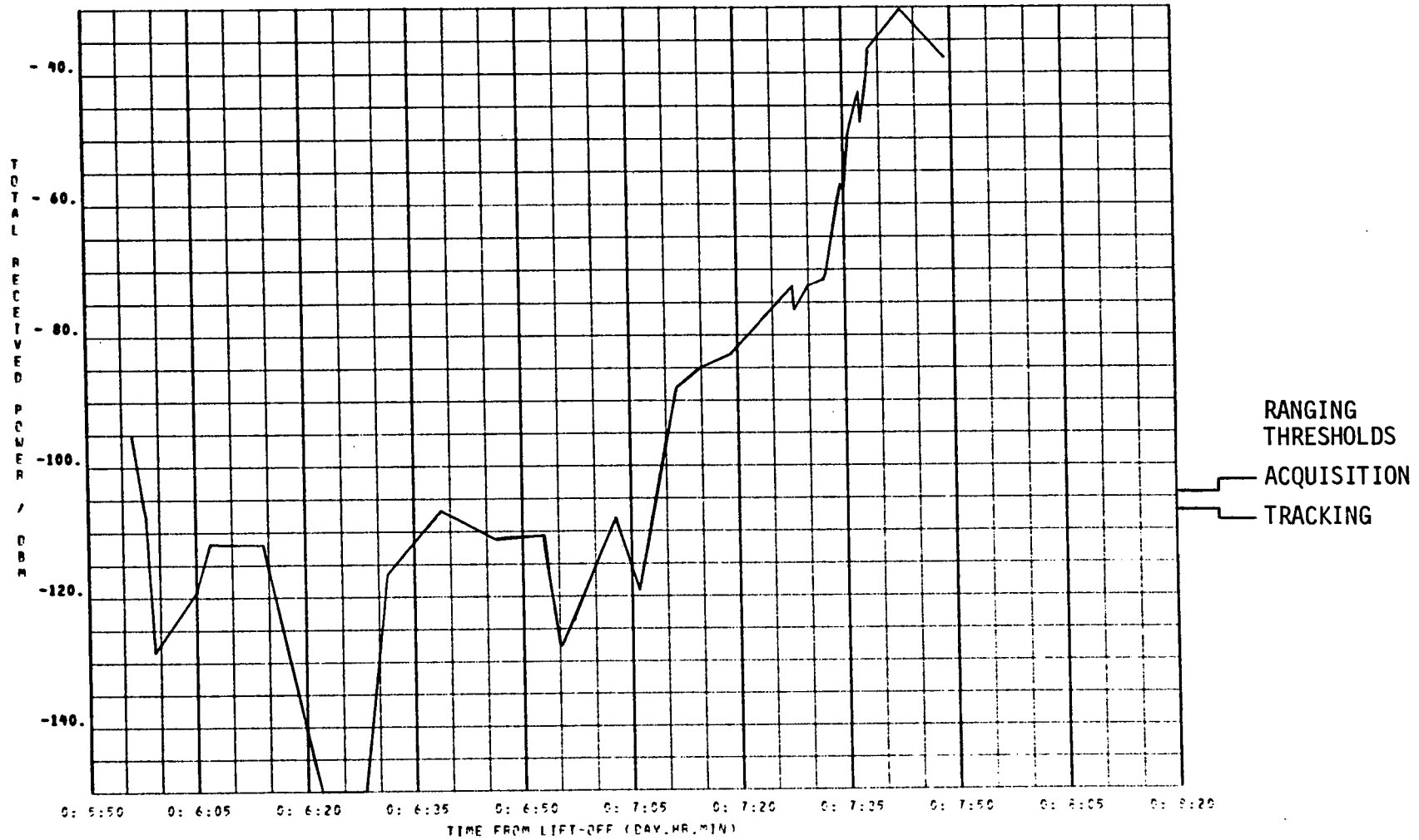
Figure 19. Minimum Received Power. - 259.7 MHz - CSM Right and SWS Helix (Early TPI)
