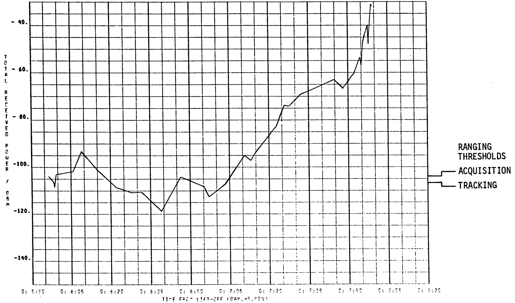
Figure 39. Maximum Received Power - 296.8 MHz - CSM Right and SWS Helix (Late TPI)
