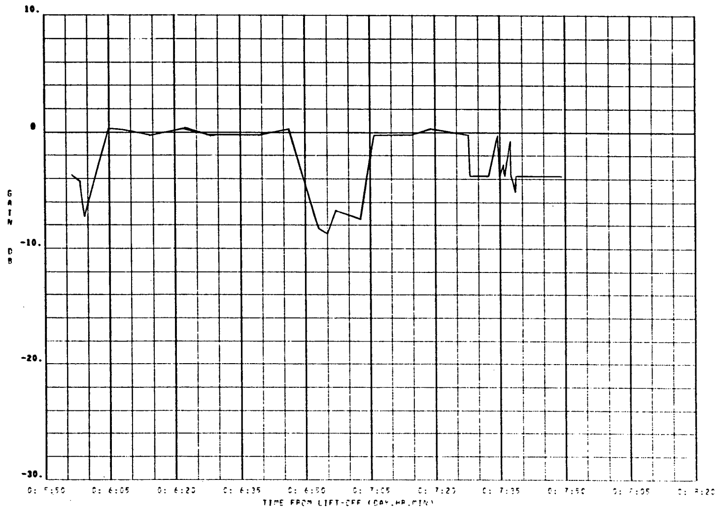
Figure 11. CSM Right Antenna Gain - 259.7 MHz (Early TPI)
