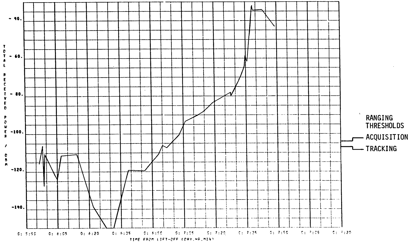
Figure 21. Minimum Received Power - 296.8 MHz - CSM Left and SWS Helix (Early TPI)
