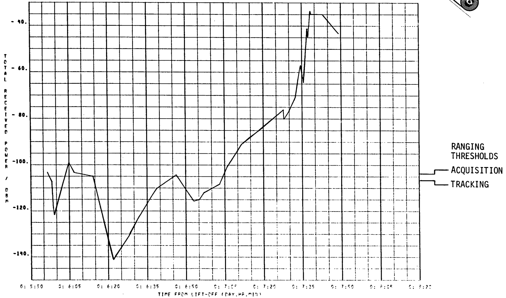
Figure 23. Minimum Received Power - 296.8 MHz - CSM Right and SWS Helix (Early TPI)
