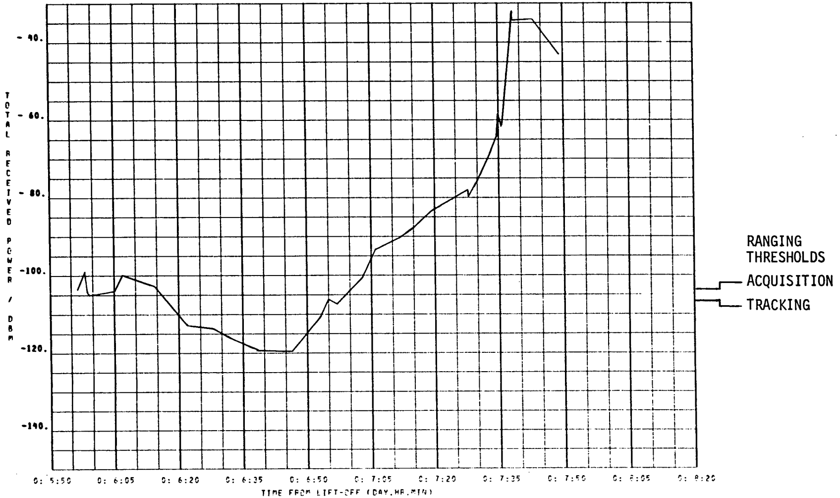
Figure 20. Maximum Received Power - 296.8 MHz - CSM Left and SWS Helix (Early TPI)
