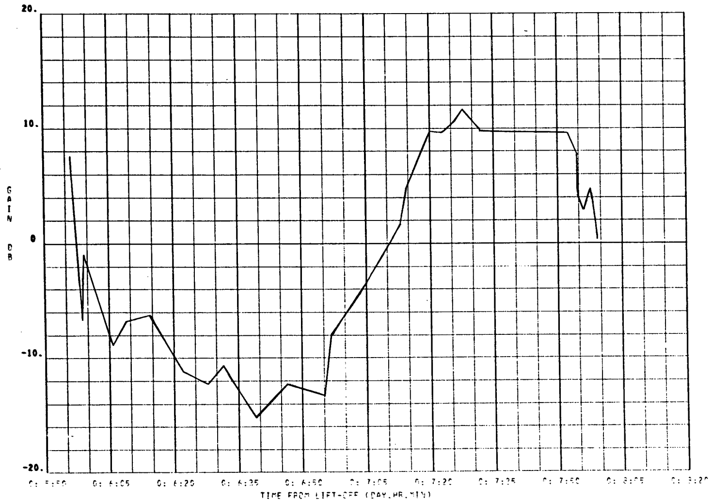
Figure 29. SWS Antenna Gain - 259.7 MHz (Late TPI)
