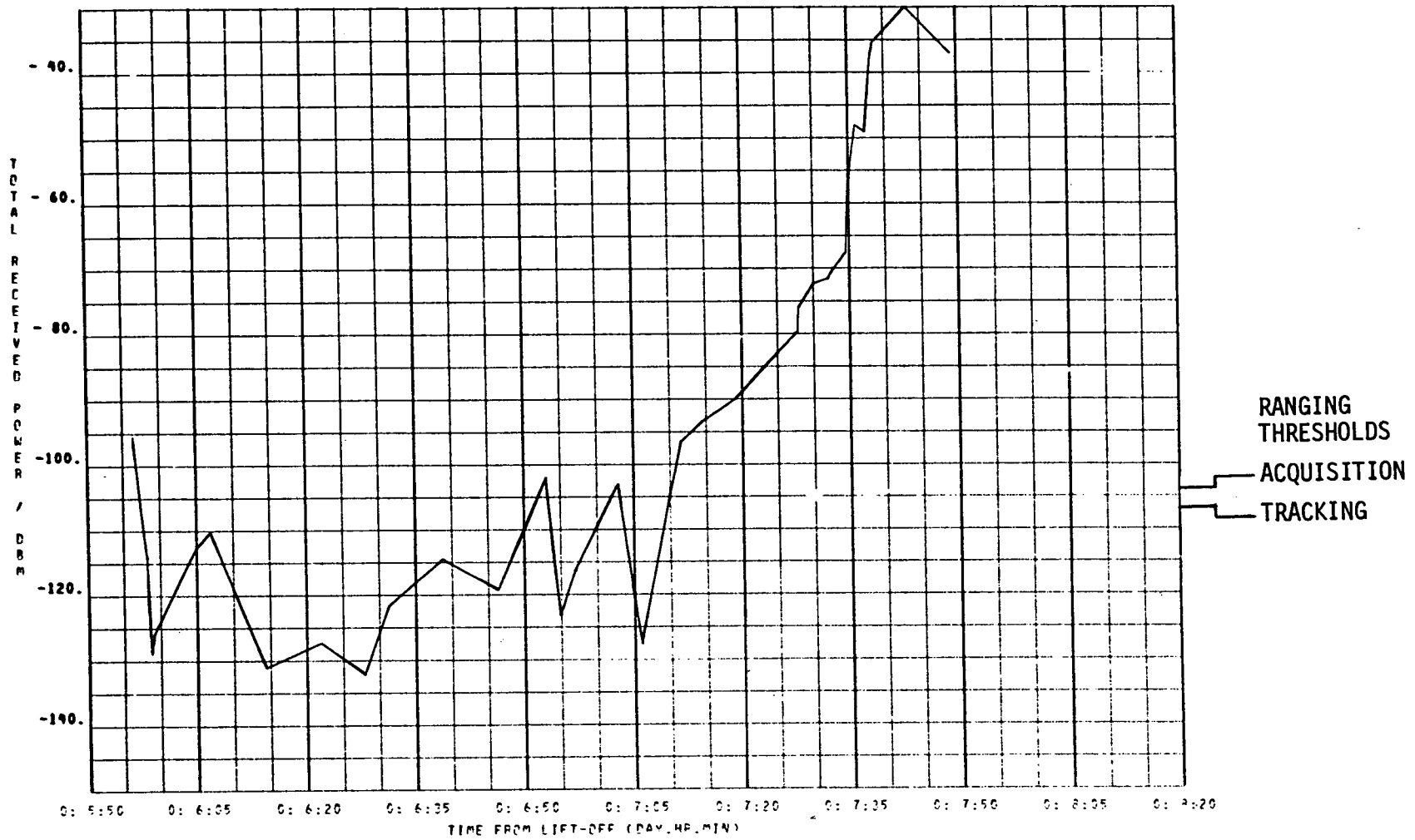
Figure 17. Minimum Received Power - 259.7 MHz - CSM Left and SWS Helix (Early TPI)
