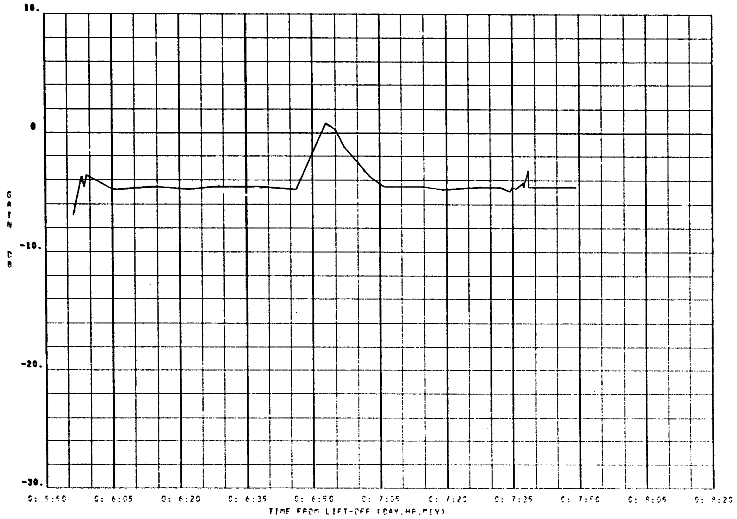
Figure 13. CSM Left Antenna Gain 296.8 MHz. (Early TPI)
