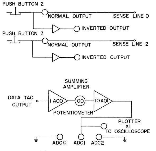
Figure A.2: Analog Computer Wiring Diagram
