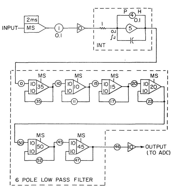
Figure 3: Analog Computer Data Tachometer Schematic
