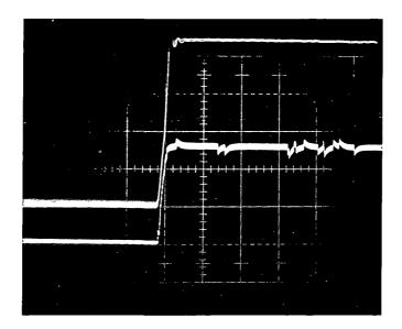
Figure 4: Analog Computer and Standard Data Tachometer Outputs
