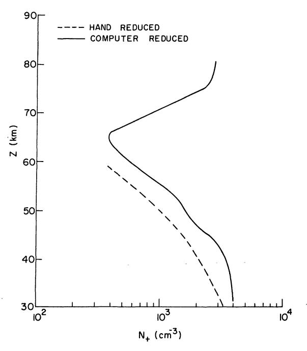
Figure 15: Smoothed Positive Ion Density Curves for 31 Jan 1972
