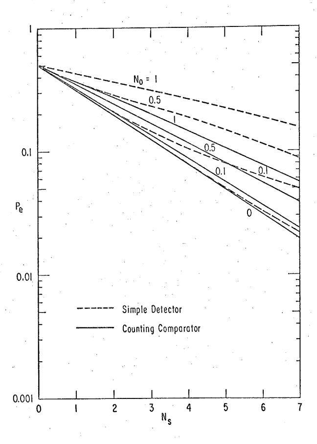
Figure 22 Average error probability  $P_e$  in binary detection vs. average number  $N_s$  for simple detector and counting comparator with square observation area  $A' = 4\sigma^2$  at  $R_0 = 1$  and  $N_0 = 0.1$ ;  $x_0/\sigma = 1$ , 2.
