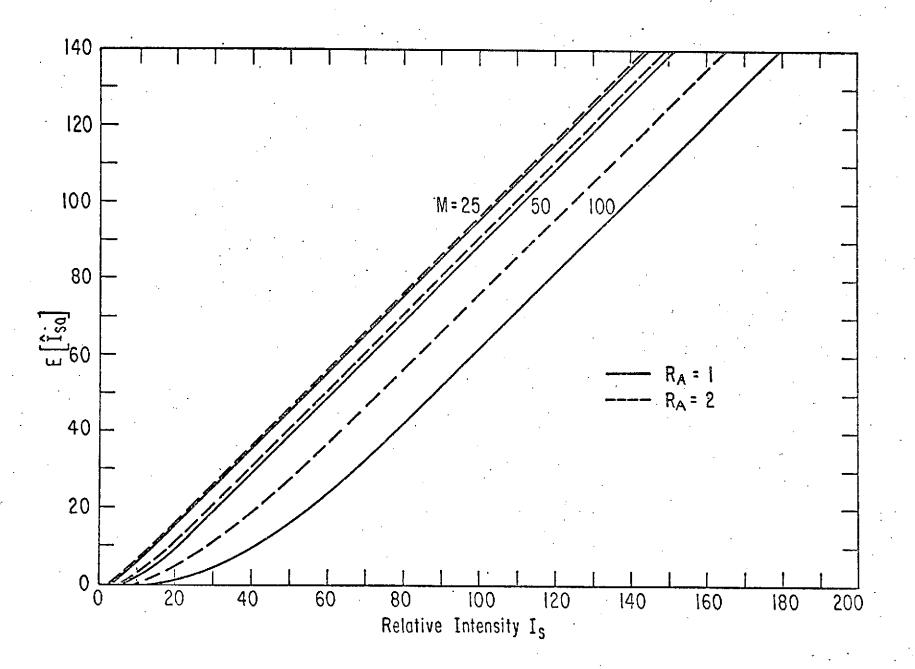
Figure 15 Mean estimate  $\hat{I}_{Sa}$  vs. relative intensity  $I_S$  for truncated Gaussian image;  $Q_0 = 10^{-2}$ , M = 100,  $\mu$  = 0.1 at  $R_A$  = 1 for time T. Curves are indexed by observation intervals T.
