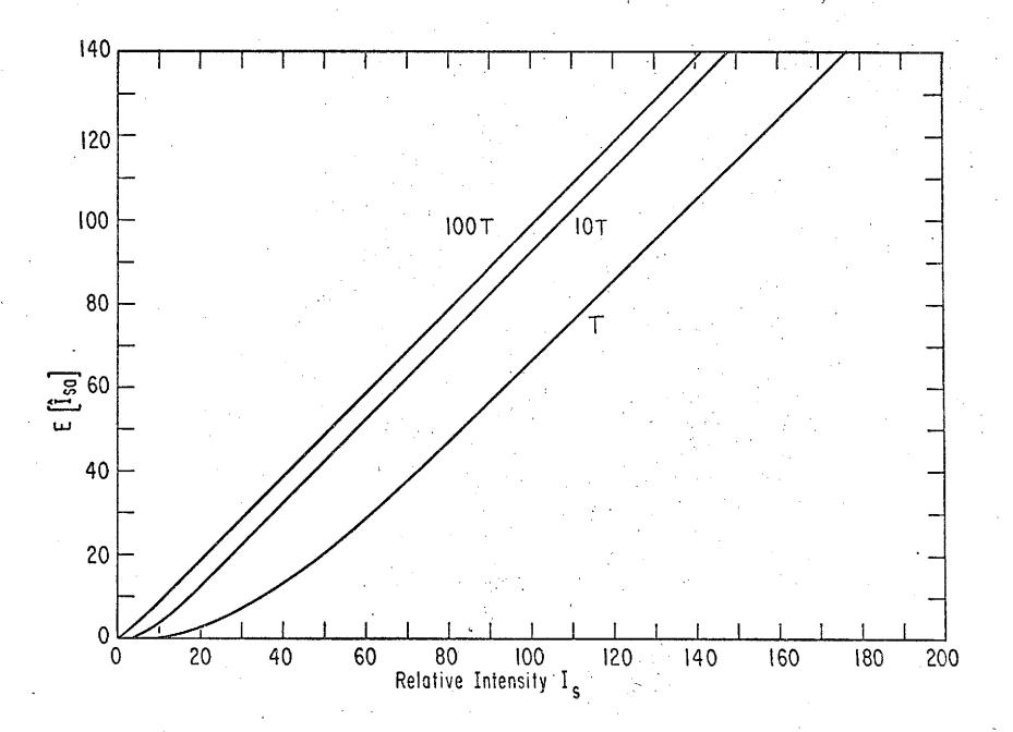
Figure 18 Error vs. mean counts  $\mu$  for parabolic image;  $Q_0 = 10^{-2}$ . Curves are indexed by parameters  $I_S$  defined in (3.47) and M.
