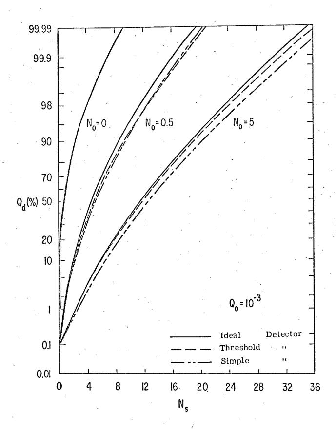
Figure 8 Probability  $Q_d$  as a function of  $N_s$  for ideal, threshold and simple detectors,  $Q_0 = 10^{-5}$  at  $N_0 = 0$ , 0.5, 5.
