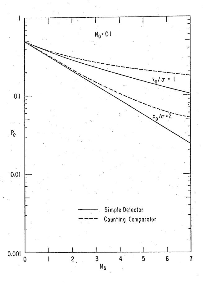
Figure 23 Average error probability  $P_e$  in binary detection vs. average number difference  $\Delta N$  for simple detector and counting comparator where  $\Delta N = \overline{n}_{T1} - \overline{n}_{T0}$  with  $\overline{n}_{Tk}$  as the mean number of photoelectrons observed from a finite area of one-half of the surface under hypothesis  $H_k$  for k=0, 1;  $\overline{n}_{T0} = 0.5$ , 1, 2.
