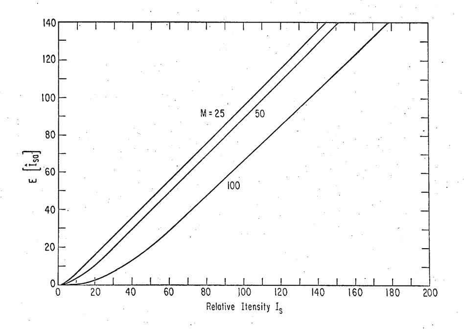
Figure 17 Mean estimate  $\hat{I}_{Sa}$  vs. relative intensity  $I_{S}$  for parabolic image:  $Q_0 = 10^{-2}$ ,  $\mu = 0.1$  at  $R_0 = 1$  for time T. Curves are indexed by observation intervals T.
