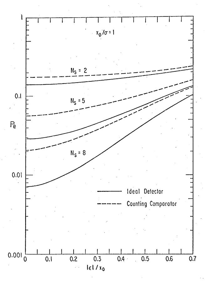
Figure 26 Average error probability  $P_e$  in binary bits detection vs. the ratio  $|\varepsilon|/x_0$  due to the mislocation of the images for the ideal detector and the counting comparator for fixed value  $N_s = 5$ ;  $x_0/\sigma = 1.5$ , 2, 4.
