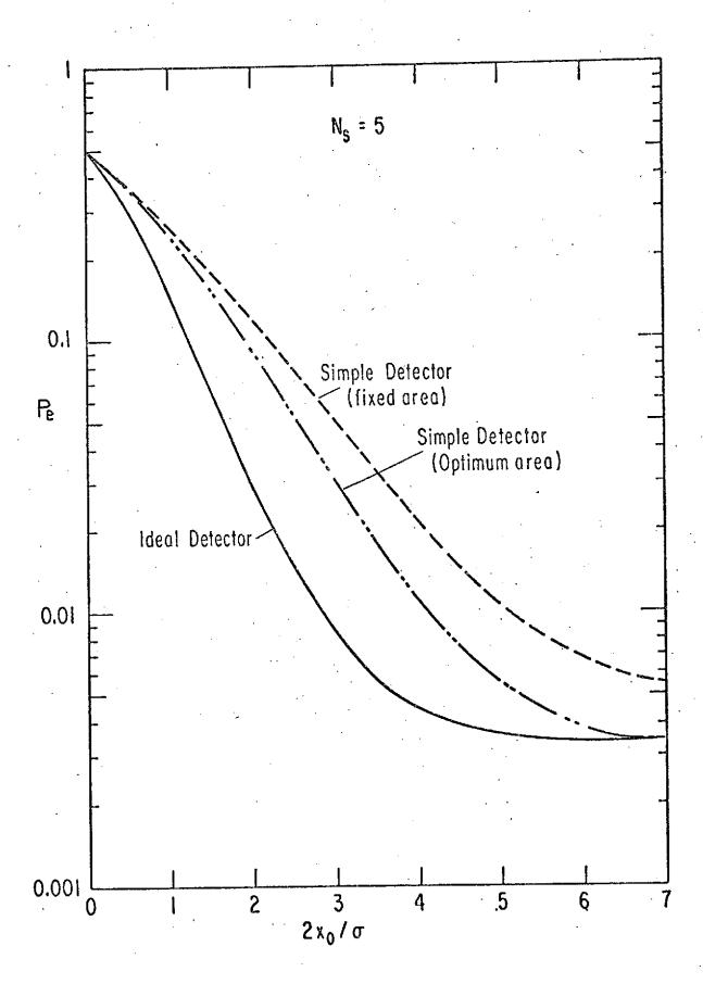
Figure 21 Average error probability  $P_e$  in binary detection vs. average number  $N_s$  for simple detector, counting comparator with square observation area  $A^1 = 4\sigma^2$  at  $R_0 = 1$  and  $x_0/\sigma = 2$ ,  $N_0 = 0$ , 0.1, 0.5, 1.
