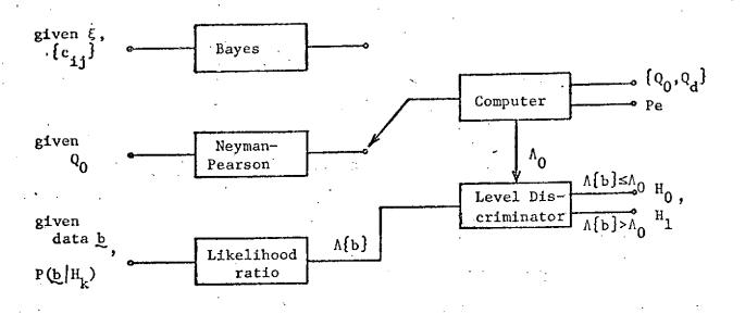
Figure 2 Block diagram of hypothesis test for binary detection.
