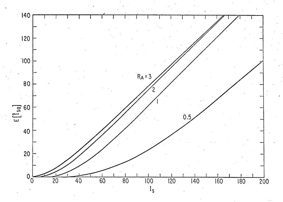
Figure 14 Mean estimate  $\hat{I}_{Sa}$  vs. relative intensity  $I_S$  for truncated Gaussian image;  $Q_0 = 10^{-2}$ ,  $\mu = 0.1$  at  $R_A = 1$  for 100 rings for time T. Curves are indexed by the parameter M defined in (3.41).
