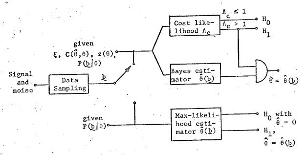
Figure 11 Block diagram for simultaneous detection and estimation of a single parameter  $\boldsymbol{\theta}$  from the signal.
