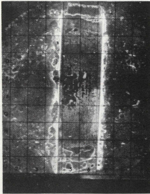
Figure 2-31A. SEM Photograph of Selected Low Strength Bondline (50X)
