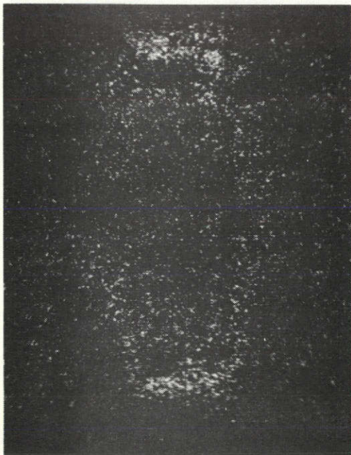
Figure 2-32C. X-Ray Map of Gold in Selected High Strength Bondline (50X)
