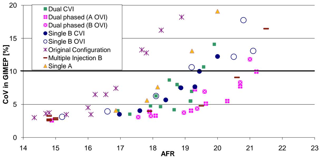
Figure 4a: Comparison of mixture response combustion sensitivity to injection strategy at KP2.
