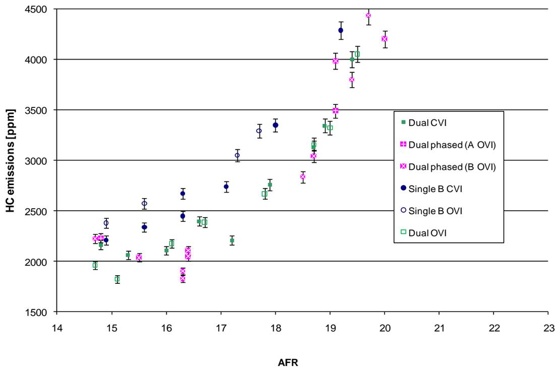
Figure 7: Comparison of ubHC emissions with air-fuel ratio for dual and single injection cases at KP2.
