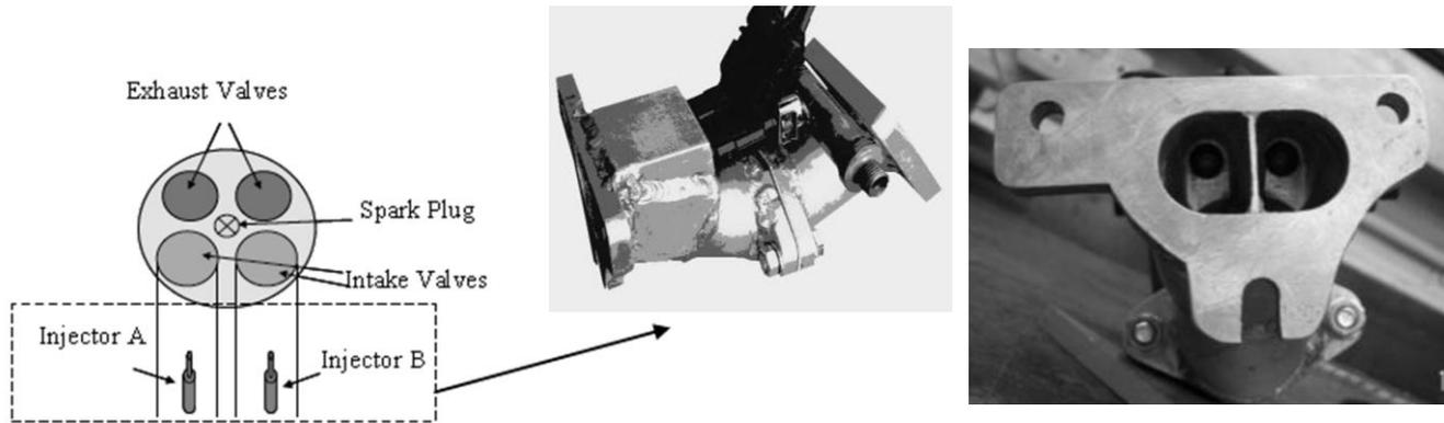
Figure 2: Single cylinder intake manifold with modified configuration incorporating twin fuel injectors and internally divided separate passages.
