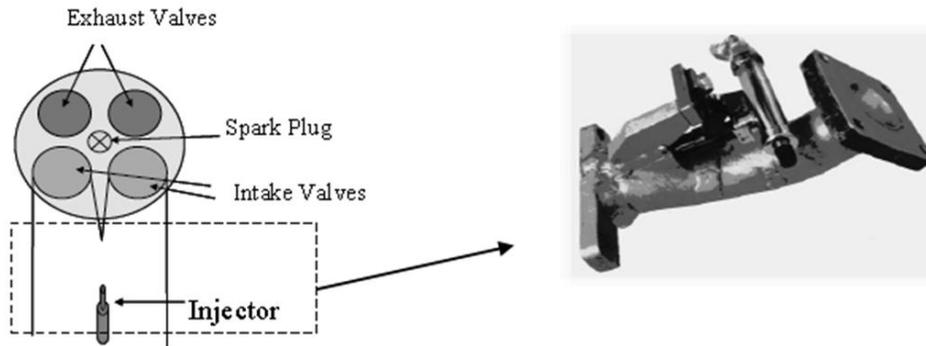
Figure 1: Single cylinder intake manifold with original configuration of a single fuel injector.
