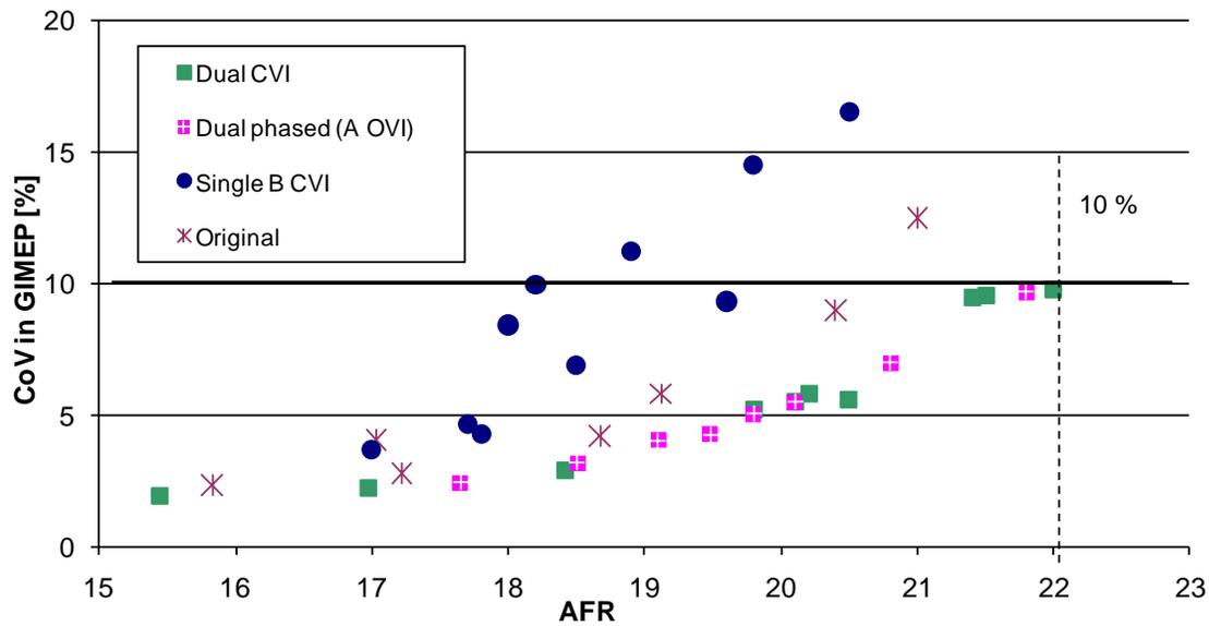
Figure 4b: Comparison of mixture response combustion sensitivity to injection strategy at KP3.
