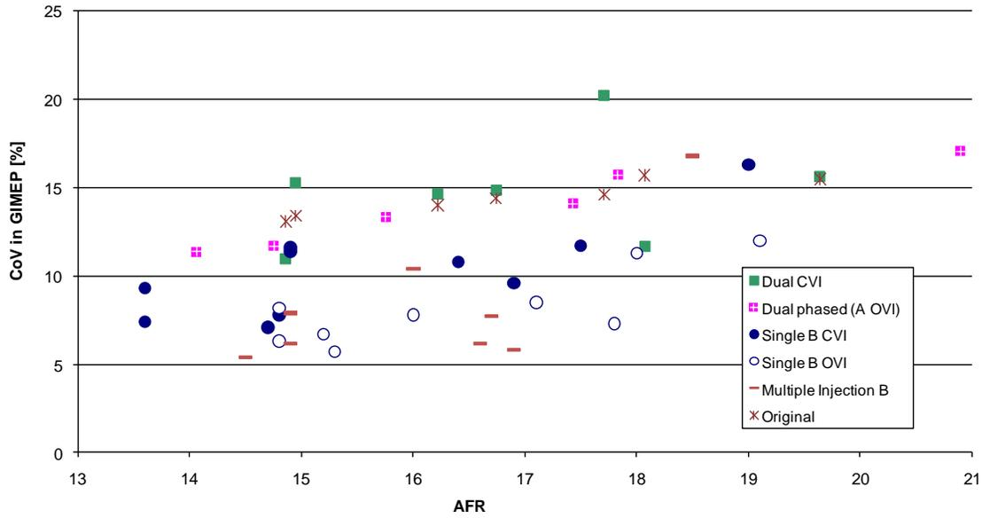
Figure 4c: Comparison of mixture response combustion sensitivity to injection strategy at KP1.
