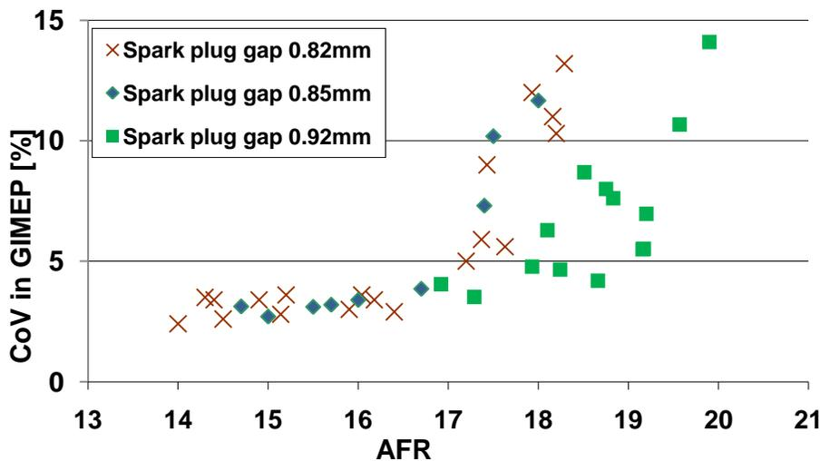
Figure 3: AFR mixture response swing using different spark plug gaps at KP 2.
