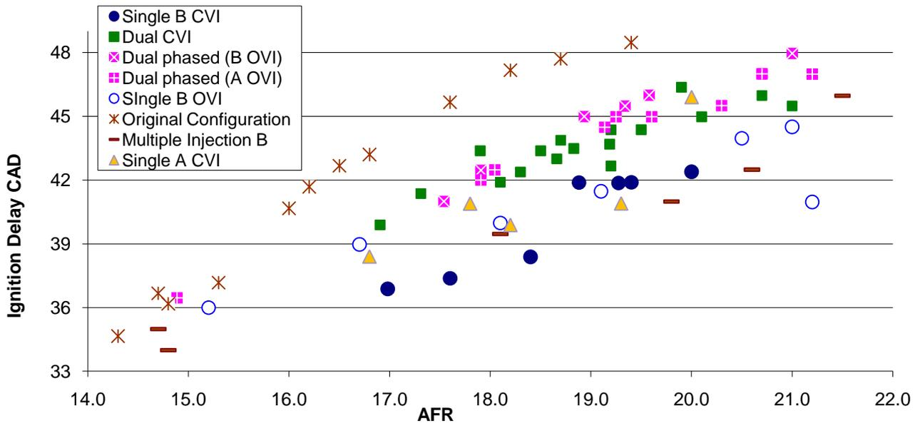
Figure 5: Ignition delay angle, defined as ignition to 10% MFB, response to AFR at KP2.
