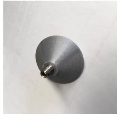
Figure 7: Backshell of Model with Epoxied Threaded Rod
