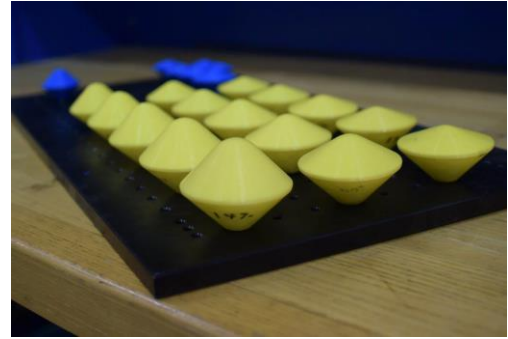
Figure 5: 3D Printed Models with Nose Cone Semi-Vertex Angles of 45,60, and 70 Degrees (L-R)
