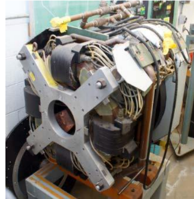
Figure 1: Magnetic Suspension and Balance System developed by MIT
