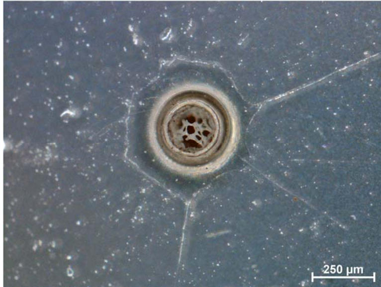
Figure 12. Optical microscope image of an impact site in the ram Al-FEP flight sample (M8-R2).
