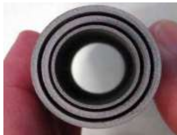
Reentrant Ti6-4 tube for a cryogenic thermal switch for the ASTRO-H Adiabatic Demagnetization Refrigerator
