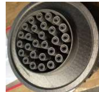
28-element Inconel 625 fuel injector
