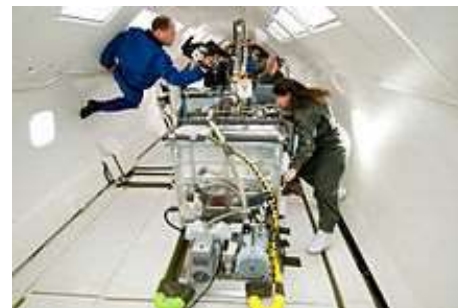
EBF 3 wire-fed system during parabolic flight testing
