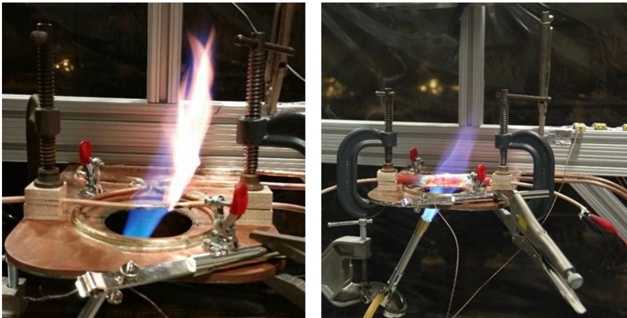
Figure 11. Fire Testing of an Antenna Cable without (left) and with (right) a Firesleeve
