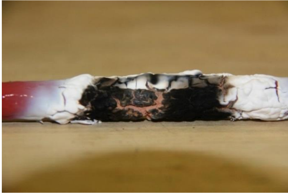
Figure 12. Firesleeve Post-Test Condition
