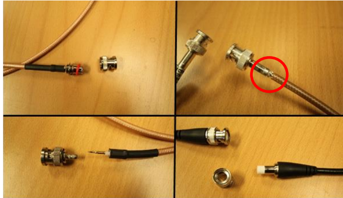
Figure 9. Antenna Cable Connector Failures from Strength Testing
