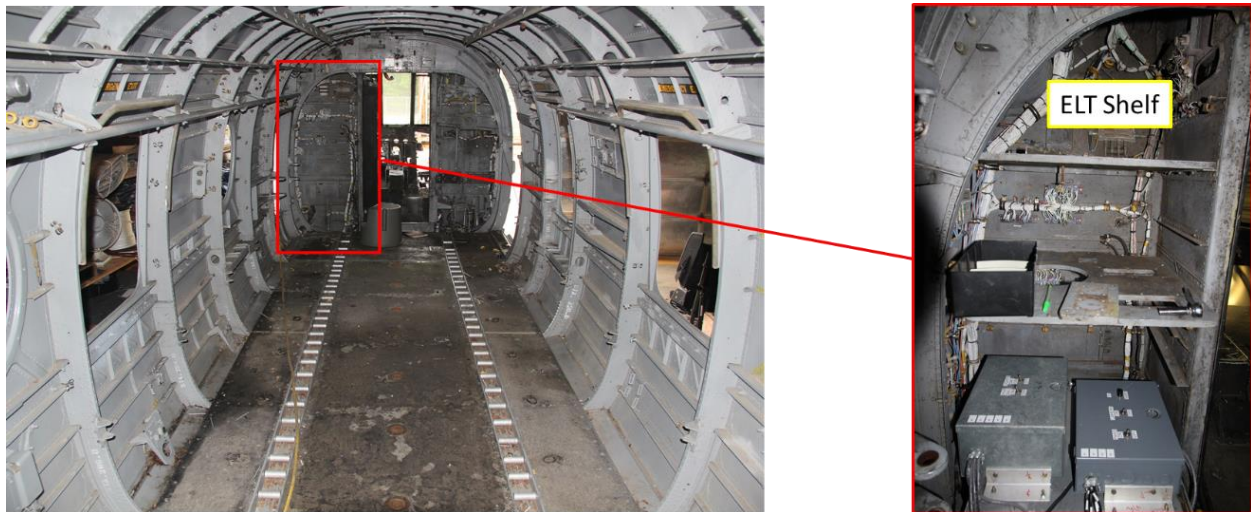
Figure 15. ELT Shelf Onboard TRACT 2
