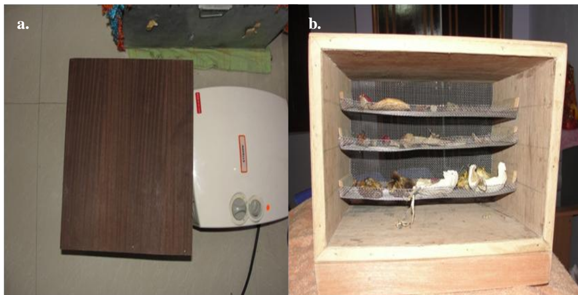
Figure 49. (a)A room heater (b) The structure constructed to dry mushrooms as a substitute of a mushroom dryer.
